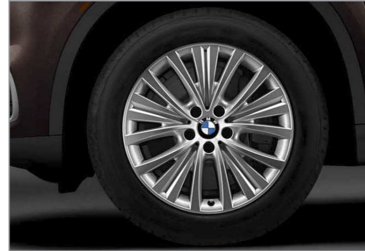
Multi Spoke light alloy wheels (Style 448) 19 x 9.0 front and rear; and 255/50 front and rear run-flat all-season tires 1,2
