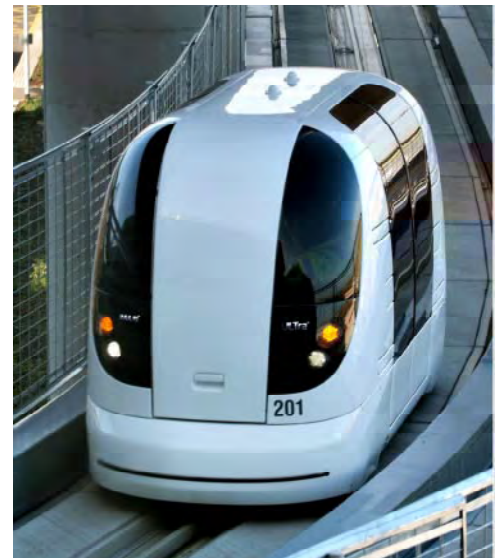
Figure B1. The ULTra PRT System Vehicle as deployed at London Heathrow Airport.
