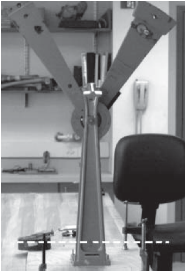
Figure 1a. Hounsfield Balanced Impact Test Machine. The pendulum on the left (outer pendulum) is slotted in the middle (and has the impact platens) such that the pendulum on the right (inner pendulum, with the specimen) can swing through it. The white dashed line indicates the location of the impact plane.
