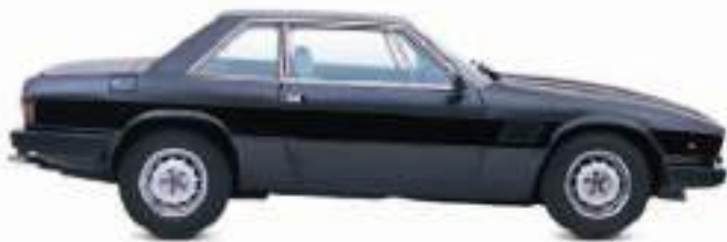
△ Maserati Kyalami 4.9 1976 Origin Italy Engine 4,930 cc, V8 Top speed 160 mph (257 km/h) When Alejandro De Tomaso took over Maserati, he developed his 1972 Ghia-designed Longchamp model into the Kyalami, with a choice of potent Maserati V8 engines.
