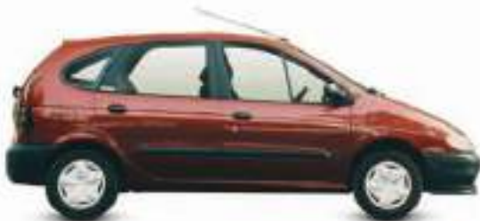
△ Renault Mégane Scénic 1996 Origin France Engine 1,598 cc, straight-four Top speed 106 mph (171 km/h)
