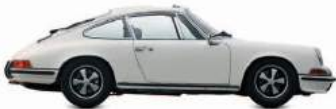
△ Porsche 911S 2.2 1970 Origin Germany Engine 2,195 cc, flat-six Top speed 144 mph (232 km/h) The 911 gained improved handling for the 1970s by moving the rear wheels back by 2.2 in (5.5 cm) and the fuel-injected S took full advantage, becoming a junior supercar.
