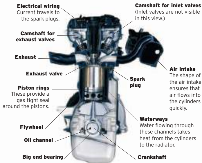
CYLINDER CROSS-SECTION
