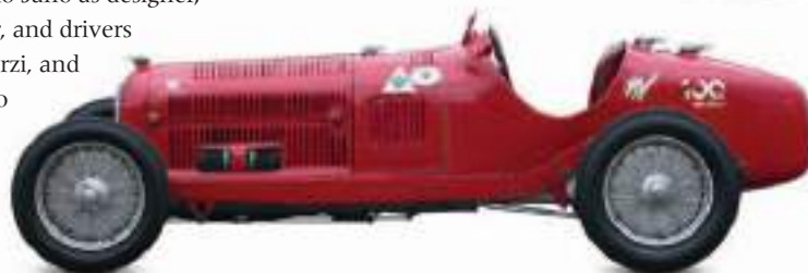
◁ Alfa Romeo Tipo B 1932 Origin Italy Engine 2,650 cc, straight-eight Top speed 140 mph (225 km/h)
