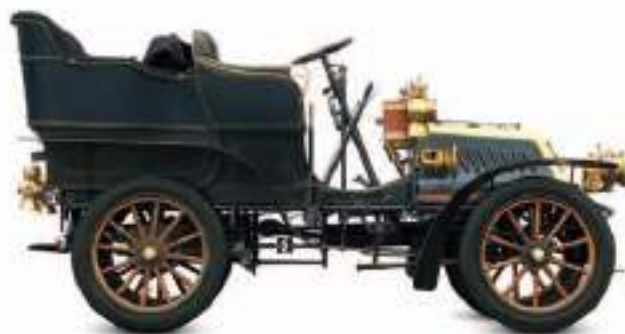
△ De Dion-Bouton 10HP Type W 1904 Origin France Engine 1,728 cc, straight-two Top speed 40 mph (64 km/h)
