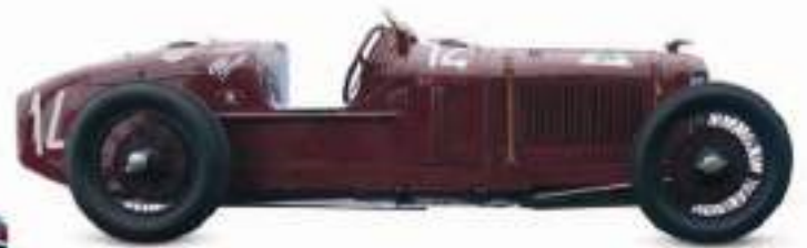
△ Alfa Romeo P2 1924 Origin Italy Engine 1,987 cc, straight-eight Top speed 123 mph (198 km/h)
