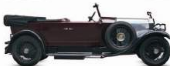
△ Rolls-Royce 20HP 1922 Origin UK Engine 3,128 cc, straight-six Top speed 65 mph (105 km/h)
