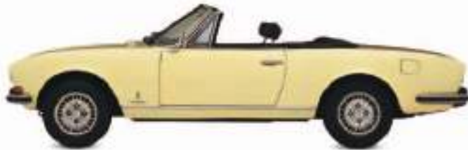
△ Peugeot 504 Cabriolet 1969 This handsome four-seater was designed and built for Peugeot by Pininfarina. There was a coupé version too; both used mechanical parts from the 504 and 604 sedans. Origin France/Italy Engine 2,664cc, V6 Top speed 110 mph (177 km/h)
