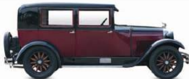
△ Essex A 1919 Origin USA Engine 2,930 cc, straight-four Top speed 65 mph (105 km/h)
