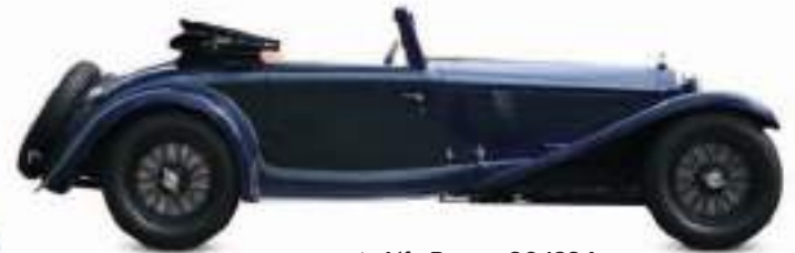
△ Alfa Romeo 8C 1934 Origin Italy Engine 2,336 cc, straight-eight Top speed 105 mph (169 km/h)
