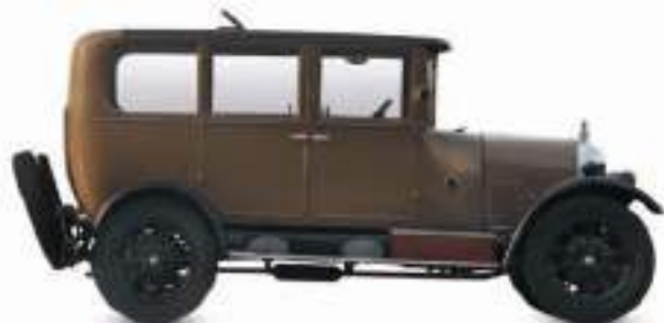
△ Morris Cowley 1927 Origin UK Engine 1,548 cc, straight-four Top speed 60 mph (97 km/h)
