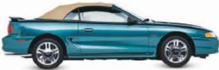
△ Ford Mustang GT 1994 Origin USA Engine 4,942 cc, V8 Top speed 136 mph (219 km/h)
