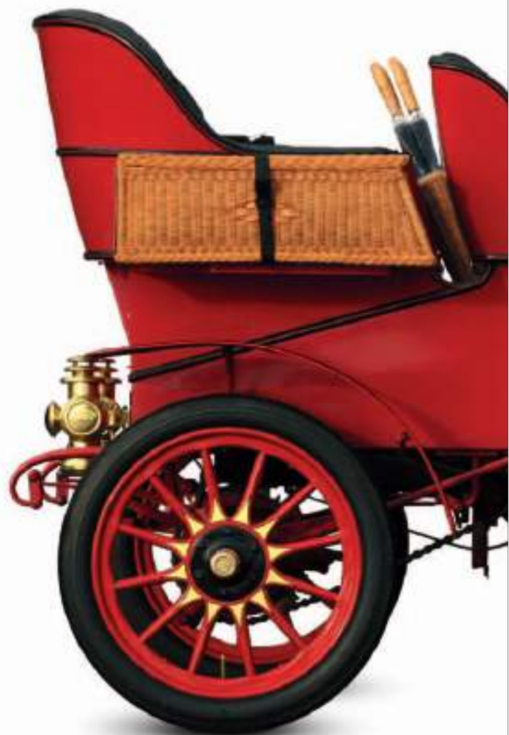
△ Cadillac Model A 1903 Origin USA Engine 1,606 cc, single-cylinder Top speed 35 mph (56 km/h)
