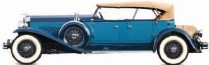
▷ Duesenberg Model J 1928 Origin USA Engine 6,882 cc, straight-eight Top speed 115 mph (185 km/h)
