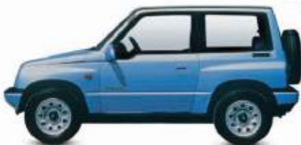
▷ Suzuki Vitara 1988 Origin Japan Engine 1,590 cc, straight-four Top speed 87 mph (140 km/h)
