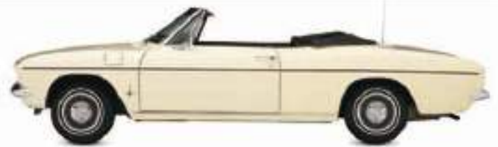
△ Chevrolet Corvair Monza 1965 Origin USA Engine 2,687 cc, flat-six Top speed 90 mph (145 km/h)
