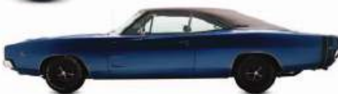
◁ Dodge Charger R/T 1968 Origin USA Engine 5,211 cc, V8 Top speed 113 mph (182 km/h)
