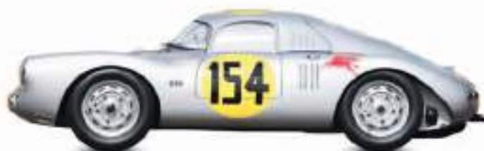
◁ Porsche 550 Coupé 1953 Origin Germany Engine 1,488 cc, flat-four Top speed 124 mph (200 km/h)
