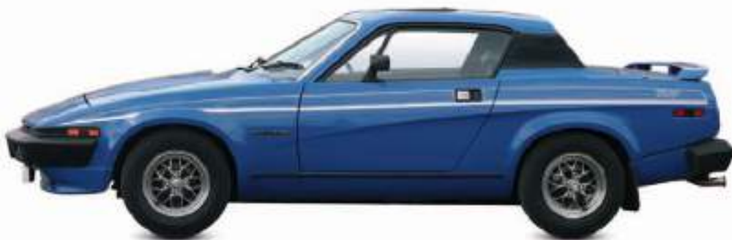
△ Triumph TR7 1975 The TR7 was built to meet anticipated safety laws, which meant a hardtop only; a convertible followed five years later. TR7 was a civilized cruiser and a big seller. Origin UK Engine 1,998 cc, straight-four Top speed 110 mph (177 km/h)
