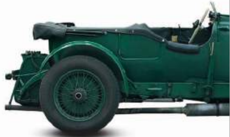
△ Cunningham touring car 1916 Exceptionally modern-looking at the time of its introduction, and boasting one of the first production V8 engines, the Cunningham attracted celebrity buyers and was produced until 1933. Origin USA Engine 7,200 cc, V8 Top speed 95 mph (153 km/h)
