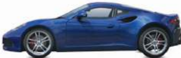
△ Artega GT 2009 Origin Germany Engine 3,597 cc, V6 Top speed 170 mph (274 km/h) Styled by Henrik Fisker, also responsible for the Aston Martin Vantage, the Artega is focused on low weight. At just 2,205 lb (1,100 kg), it is light for a supercar.
