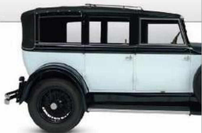
◁ Spyker C4 All-weather Coupé 1921 Origin Netherlands Engine 5,741 cc, straight-six Top speed 80 mph (129 km/h)
