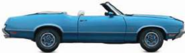
△ Oldsmobile 442 1970 Origin USA Engine 7,456 cc, V8 Top speed 120 mph (193 km/h)
