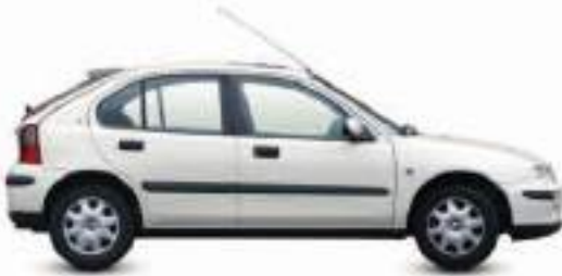
△ Rover 25 VVC 1999 Origin UK Engine 1,796 cc, straight-four Top speed 127 mph (204 km/h)
