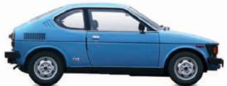
△ Suzuki SC100 Coupé 1978 Origin Japan Engine 970 cc, straight-four Top speed 76 mph (122 km/h) Suzuki sold 894,000 rear-engined "Whizzkids," mainly on looks—they were cramped for four and had poor performance. The Mini was roomier and more nimble.
