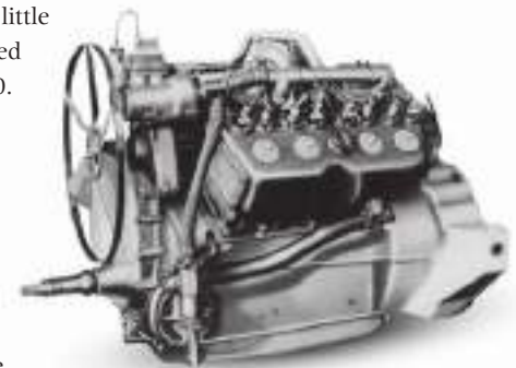
The first mass-produced V8 engine
