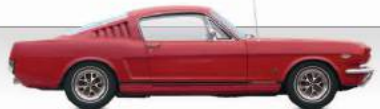
△ Ford Mustang Fastback 1965 Origin USA Engine 4,727 cc, V8 Top speed 116 mph (187 km/h)
