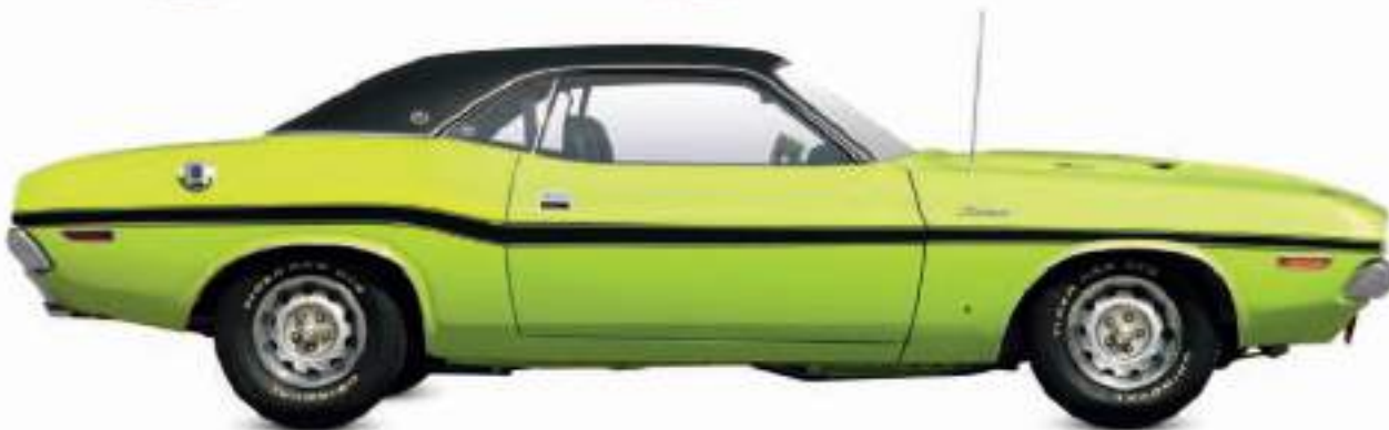
◁ Dodge Challenger R/T 440 1970 Origin USA Engine 6,276 cc, V8 Top speed 114 mph (183 km/h)
