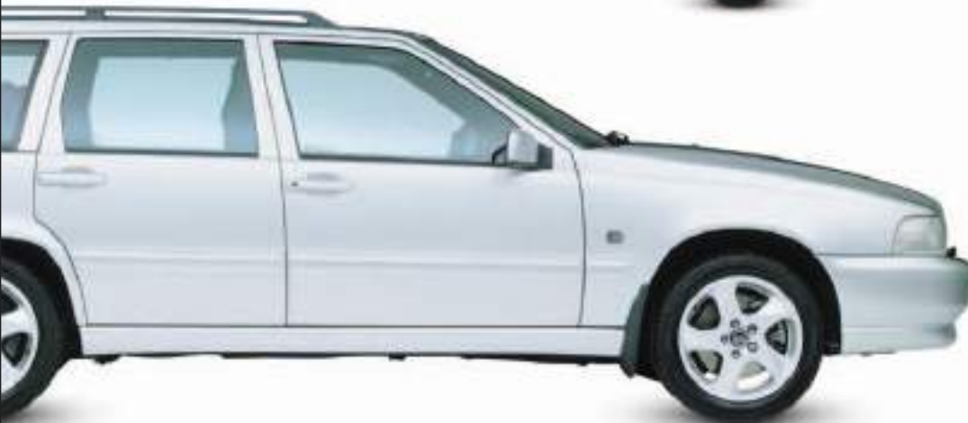
△ Volvo V70 T5 1997 Origin Sweden Engine 2,319 cc, straight-five Top speed 152 mph (245 km/h)
