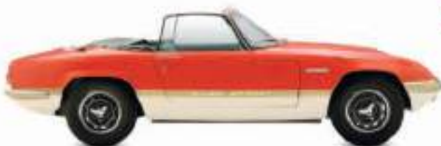
△ Lotus Elan Sprint 1971 The fifth, final, and finest incarnation of Colin Chapman's benchmark sports car, this car had superb road manners matched by 126 bhp of power, a five-speed gearbox, and spiffy livery. Origin UK Engine 1,558 cc, straight-four Top speed 120 mph (193 km/h)
