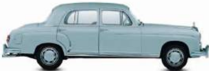
△ Mercedes-Benz 220 1954 Mercedes' first monocoque construction sedan arrived in four-cylinder form in 1953; the more powerful six-cylinder version joined it in 1954. Sturdy and well built, both sold well.
