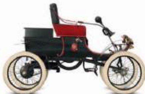
△ Oldsmobile Curved Dash 1901 Origin USA Engine 1,564 cc, single-cylinder Top speed 20 mph (32 km/h)
