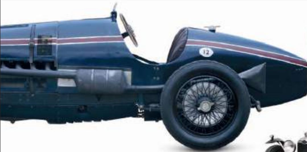
△ Delage V12 1923 Origin France Engine 10,600 cc, V12 Top speed 143 mph (230 km/h)
