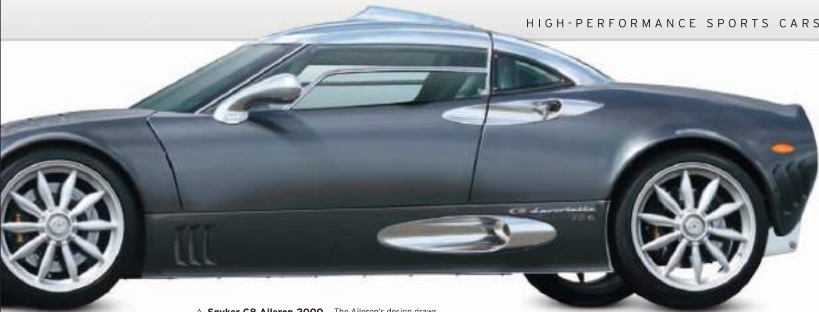
△ Spyker C8 Aileron 2000 Origin Holland Engine 4,163 cc, V8 Top speed 186 mph (299 km/h) The Aileron's design draws heavily from the company's aviation past, and even the spokes of the steering wheel are ex-propeller blades.
