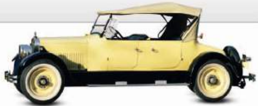
△ Cunningham touring car 1916 Exceptionally modern-looking at the time of its introduction, and boasting one of the first production V8 engines, the Cunningham attracted celebrity buyers and was produced until 1933. Origin USA Engine 7,200 cc, V8 Top speed 95 mph (153 km/h)
