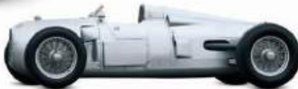
△ Auto Union Type D 1938 Origin Germany Engine 2,990 cc, V12 Top speed 205 mph (330 km/h)
