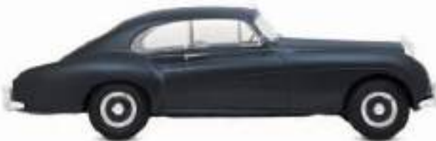
△ Bentley R-type Continental 1952 Origin UK Engine 4,566cc, straight-six Top speed 120 mph (193 km/h) Rolls-Royce finally cashed in on subsidiary Bentley's sporting heritage with this magnificent coachbuilt Grand Touring sedan, the epitome of luxury and speed.
