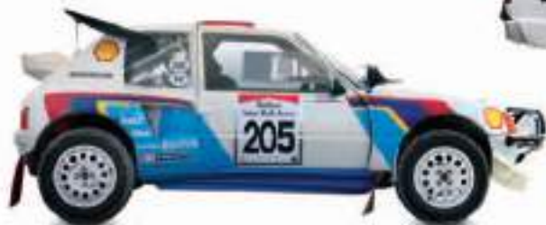
△ Peugeot 205 T16 Evo 2 1985 Origin France Engine 1,775 cc, straight-four Top speed 155mph (249 km/h)
