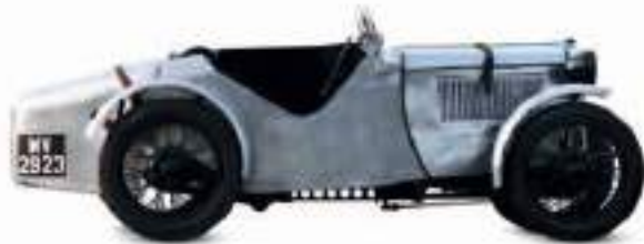
△ Austin Seven Ulster 1930 Origin UK Engine 747 cc, straight-four Top speed 80 mph (129 km/h)
