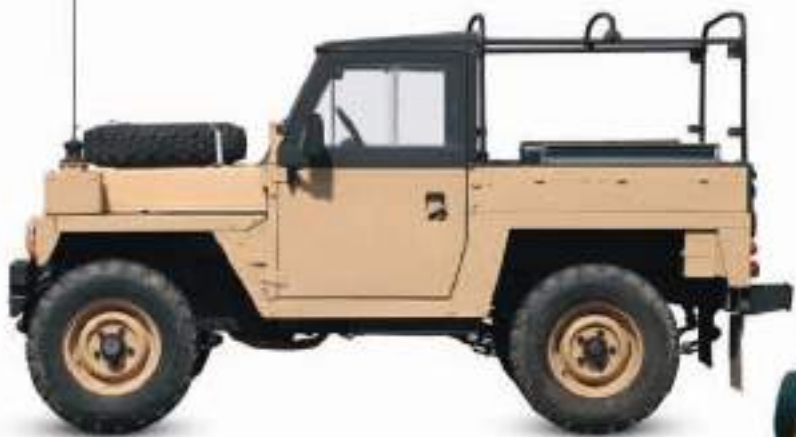
△ Land Rover 88 SIII 1971 Origin UK Engine 2,286 cc, straight-four Top speed 68 mph (109 km/h)
