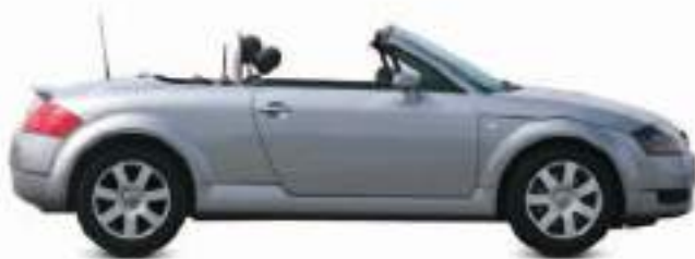
△ Audi TT Roadster 1999 Origin Germany Engine 1,781 cc, straight-four Top speed 138 mph (222 km/h)
