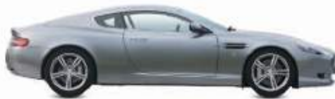
◁ Aston Martin V8 Vantage convertible 2005 Origin UK Engine 4,735 cc, V8 Top speed 180 mph (290 km/h)
