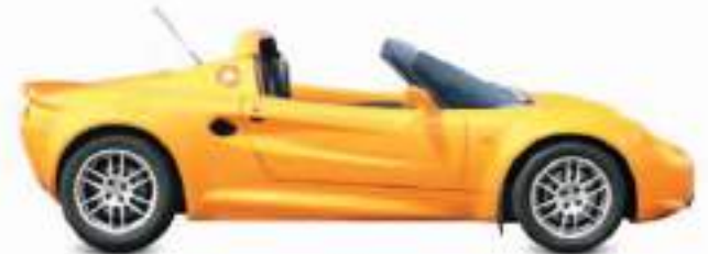
△ Lotus Elise 1996 Using a Rover K-series engine in an extruded aluminum chassis with fiberglass body, the Elise weighs just 1,599 lb (725 kg), giving superb handling and performance. Origin UK Engine 1,796 cc, straight-four Top speed 124 mph (200 km/h)
