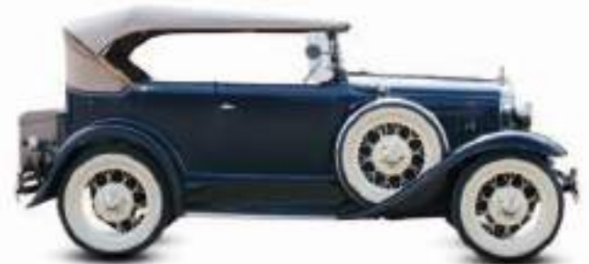
Origin USA Engine 3,285 cc, straight-four Top speed 60 mph (97 km/h)
