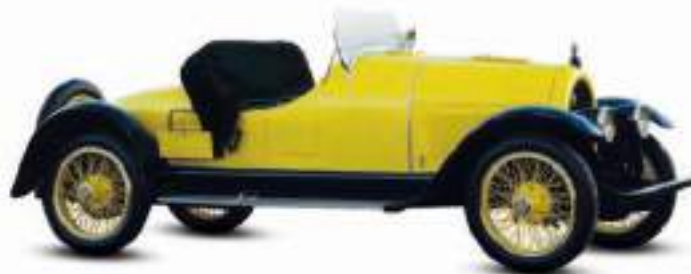
◁ Kissel straight-eight Speedster 1927 Origin USA Engine 4,670 cc, straight-six Top speed 78 mph (125 km/h)
