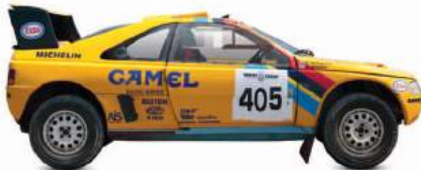
▷ Peugeot 405 T16 GR 1986 Origin France Engine 1,905 cc, straight-four Top speed 155mph (249 km/h)
