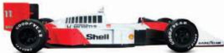
△ McLaren-Honda MP4/4 1988 Origin UK Engine 1,496 cc, V6 Top speed 210mph (338 km/h)
