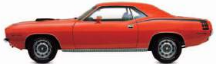
▷ Plymouth Hemi 'Cuda 1970 Origin USA Engine 7,210 cc, V8 Top speed 130 mph (209 km/h)
