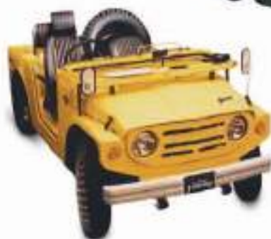
▷ Suzuki Jimny LJ10 1970 Origin Japan Engine 359 cc, straight-two Top speed 47 mph (76 km/h)
