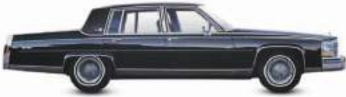
△ Cadillac Fleetwood Brougham 1980 Origin USA Engine 6,037 cc, V8 Top speed 104 mph (167 km/h)
