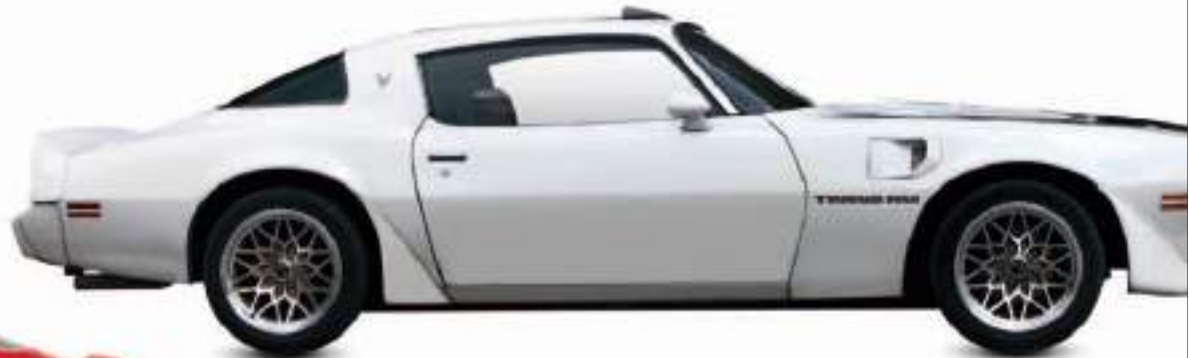
△ Pontiac Trans Am 1975 Origin USA Engine 6,556 cc, V8 Top speed 118 mph (190 km/h)
