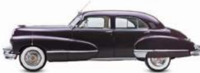
△ Cadillac Fleetwood 60 Special 1947 Origin USA Engine 5,670 cc, V8 Top speed 90 mph (145 km/h)
