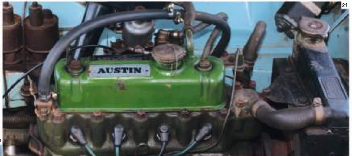
20. Hood-release catch 21. Transverse A-series engine 22. Clutch has hydraulic actuation 23. Battery and spare tire in trunk
