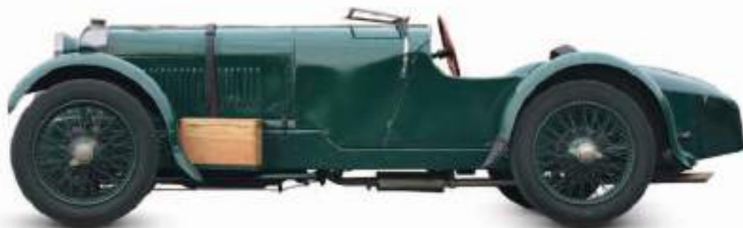
△ Alvis FWD 1928 The first front-wheel-drive, all-independently sprung sports car was too unconventional for its time to sell well. Still, it had great success on the race track.
