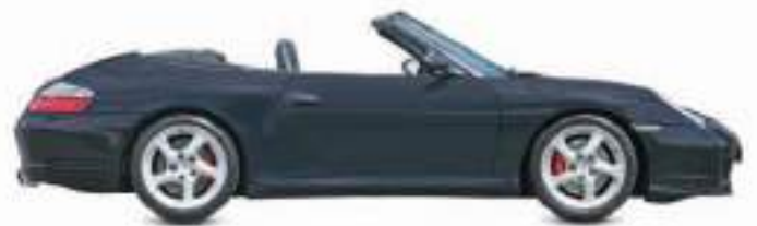
△ Porsche 911 2005 Origin Germany Engine 3,800 cc, flat-six Top speed 180 mph (290 km/h) Unofficially referred to as the 997, this is the spiritual descendant of the original 911 and still has its engine hanging out the back.
