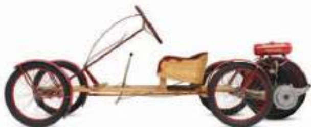
△ Briggs & Stratton Flyer 1919 Lawnmower engine maker Briggs & Stratton sold the Flyer until 1925. At $125, it was the cheapest new car ever. A motorized fifth wheel lowered to drive the flexible wood chassis.
