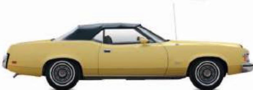
▷ Mercury Cougar 1973 Origin USA Engine 7,030 cc, V8 Top speed 125 mph (201 km/h)
