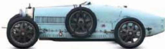
▷ Bugatti Type 35C 1926 Origin France Engine 1,991 cc, straight-eight Top speed 125 mph (201 km/h)
