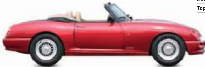
△ MG RV8 1992 The car MG should have built 25 years earlier finally entered limited production in the 1990s, with a pumped-up MGB bodyshell, Rover V8 engine, and leather trim. Origin UK Engine 3,946 cc, V8 Top speed 136 mph (219 km/h)
