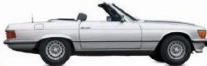
△ Mercedes-Benz 350SL 1971 An all-new SL for the 1970s, this car shared suspension hardware with the S-Class limousine. Powerful, fast, and stylish, it had a standard hardtop for winter. Origin Germany Engine 3,499 cc, straight-six Top speed 126 mph (203 km/h)
