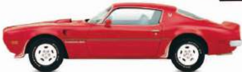
▽ Pontiac Firebird Trans Am 1973 Origin USA Engine 7,459 cc, V8 Top speed 132 mph (212 km/h)
