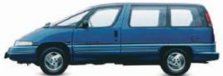
△ Pontiac Trans Sport 1989 Origin USA Engine 3,135 cc, V6 Top speed 107 mph (172 km/h)
