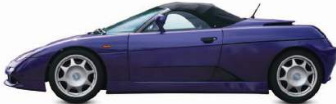
△ De Tomaso Guarà Spider 1994 More commonly sold as the Coupé or Barchetta (just five Spiders were built), this was the last project of founder Alejandro de Tomaso and used BMW running gear. Origin Italy Engine 3,982 cc, V8 Top speed 170 mph (274 km/h)
