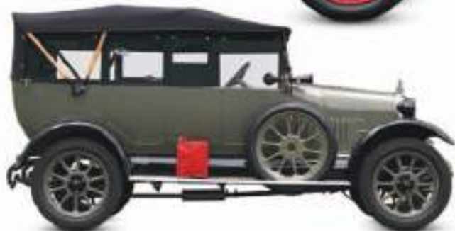
△ Morris Oxford 1919 Origin UK Engine 1,548 cc, straight-four Top speed 60 mph (97 km/h)
