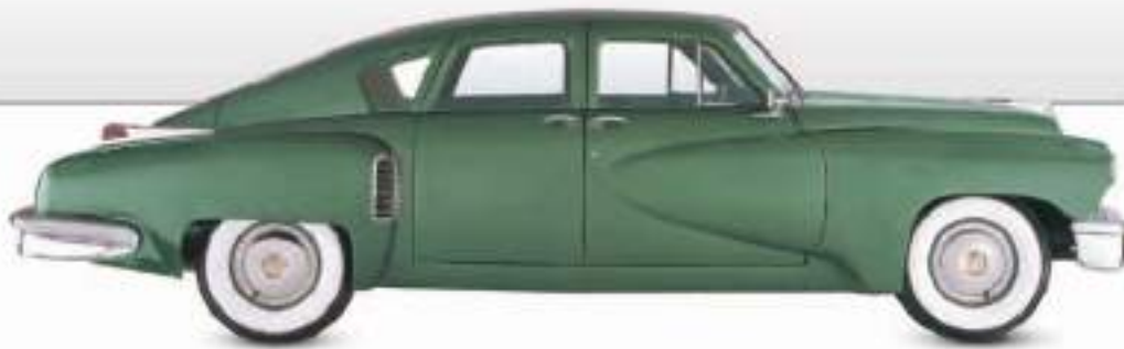
◁ Tucker 48 1948 Origin USA Engine 5,475 cc, flat-six Top speed 131mph (211 km/h)
