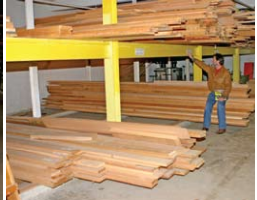
Sitka spruce is used to build aircraft and organs with aircraft getting a much higher grade.
