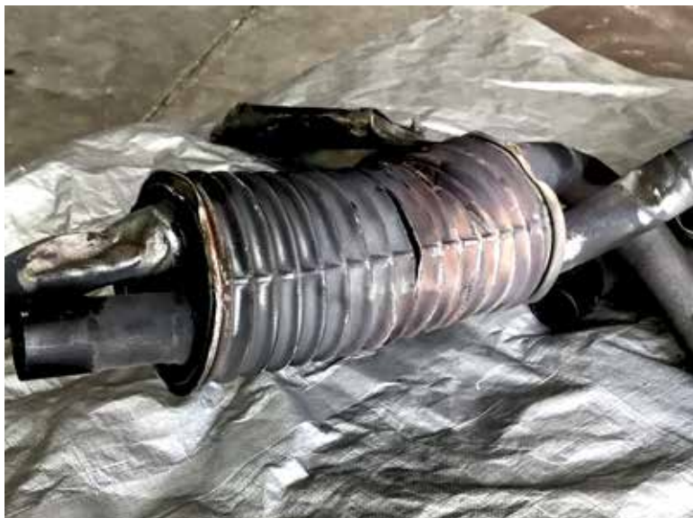
A crack in the muffler underneath the heat shroud caused exhaust to enter the cabin, resulting in carbon monoxide poisoning.
