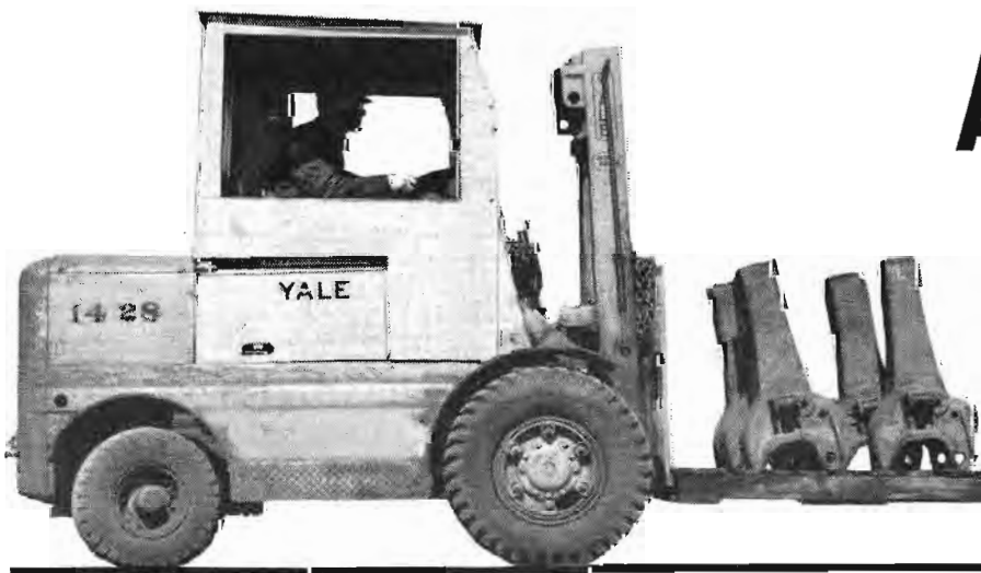
Above: Many items of material, such as this skid load of car couplers weighing 1200 pounds, require careful balancing on the fork of the lift truck to prevent their toppling off and endangering other employees. Mr. Leo watches closely as the load leaves the ground.
