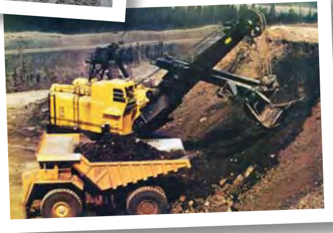
One of the best-selling modern-era electric mining shovels emerged in 1968. It was the P&H 2800 Mark II. P&H 2800-class shovels remain a highly sought-after loading tool 40 years later.
