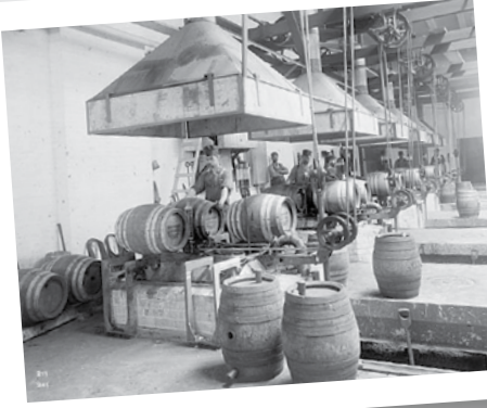
Milwaukee beer breweries were among the early customers for products from Pawling & Harnischfeger, suppliers of "pitching" or beer keg sealing machines including several built for the Joseph Schlitz Brewery.
