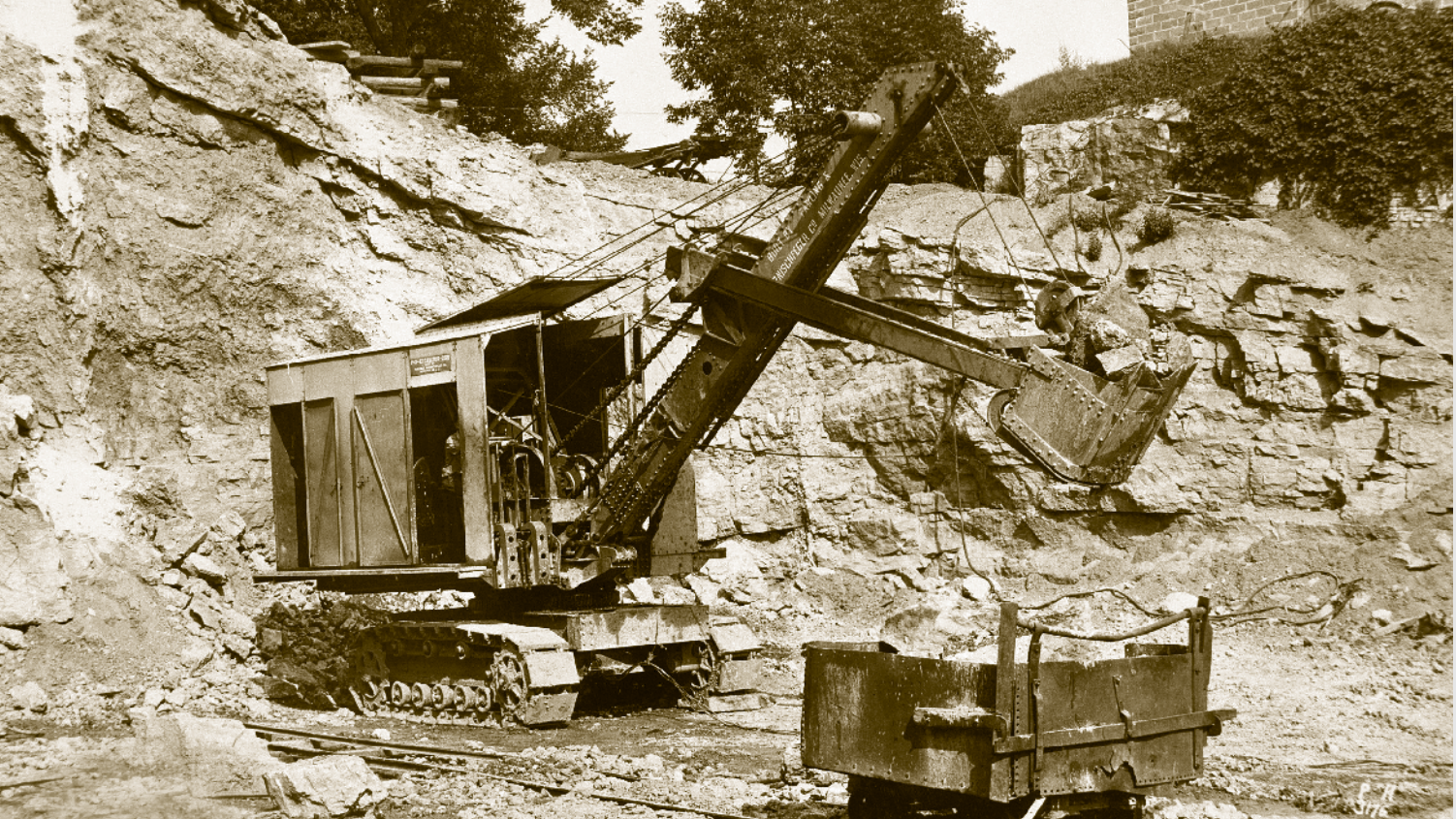
Powered by the customer's choice of a Waukesha gasoline engine, a Buda diesel engine, or a P&H electric motor, the P&H® 206 excavator introduced in 1920 would be the first in a long line of high performance digging machines bearing the P&H trademark.
