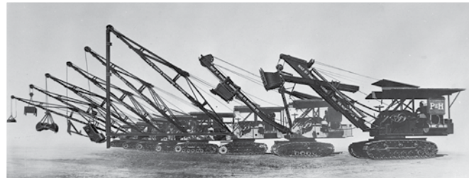
In 1927, P&H® 300 'convertibles' joined the P&H product line. The customer could choose from many functional options including power shovel, dragline, "Skim-Scoop," pile driver, clamshell and magnet crane attachments.
