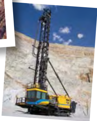
P&H Mining Equipment acquired the Gardner-Denver line of blast hole drilling rigs in 1991. A customer-driven continuous improvement program over ensuing years would result in high-performance models including the P&H® 320XPC heavy-duty drill.
