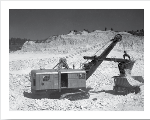
For increased strength, reduced working weight and bigger payloads, P&H began applying all-welded design to its product line starting around 1932. P&H® 1200WL shovels equipped with Ward-Leonard DC drive controls were among the first P&H all-welded digging machines.
