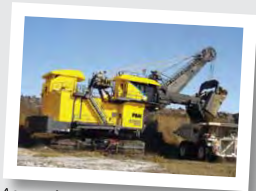
A successful roll-out of AC-drive P&H 4100BOSS shovels in 2007 launched further AC-drive shovel offerings including AC P&H® 4100XPCs in 2010.
