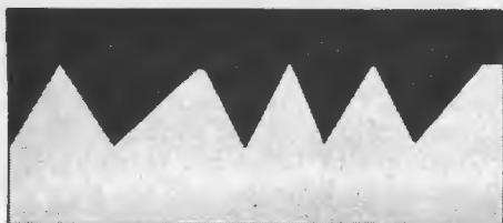
Figure No 35 If lacquer color is now applied over this surface, swelling of the primer surface will bring it back to its level at the time of sanding or slightly higher making for thin coats of lacquer over the deep fills.
