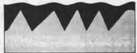
Figure No. 34. If sanded level before all solvents have evaporated further evaporation of solvents will cause a shrinkage leaving furrows over sand marks in metal.
