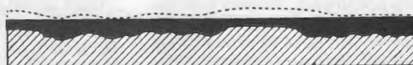
Fig 26—Sanding levels off high spots, producing a flat, smooth surface. If not dry when sanded, further shrinking over deep fills produces uneven surface and shows file marks.
