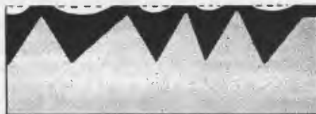
Figure No 33 Primer surfacer applied over sanded metal simulates the contours of the metal, shrinkage being more over the deeper fills.
