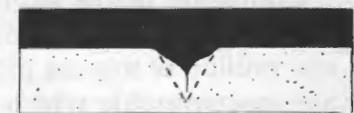
Figure 22—The solvents in the fresh coat of lacquer cause swelling in the freshly exposed parts of the scratch.
