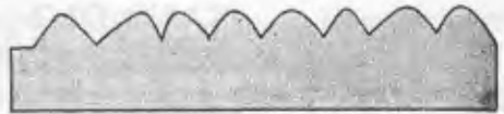
Figure No 32 Light scuffing with No 150 paper will remove combs and will round tops of ridges eliminating much trouble with sand scratches.
