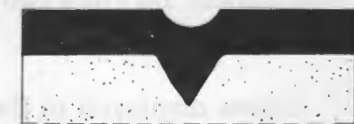
Figure 23—The swelling recedes after all of the solvents have evaporated and the new finish shrinks leaving furrows similar to the old scratches.
