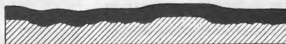
Fig 25—Same metal coated with Primer-Surfacer. Surface of undercoat follows approximate contours of original metal when thoroughly dry.
