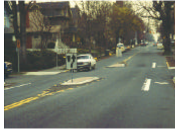
FIGURE V-12. SIGNING AND MARKING OF CENTER ISLANDS ON COLLECTOR ROADS
