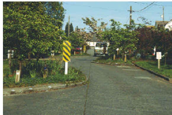
FIGURE V-17. TYPE 3 OBJECT MARKERS ON CURB EXTENSIONS AND EDGE ISLANDS
