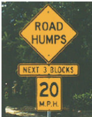
FIGURE V-1. ADVANCE WARNING SIGN WITH RIDERS
