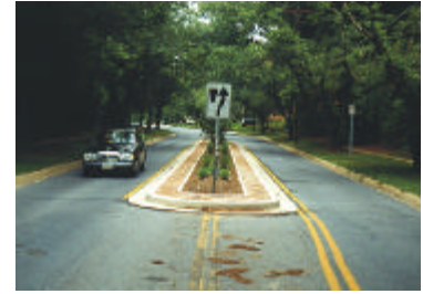
FIGURE V-12. SIGNING AND MARKING OF CENTER ISLANDS ON COLLECTOR ROADS
