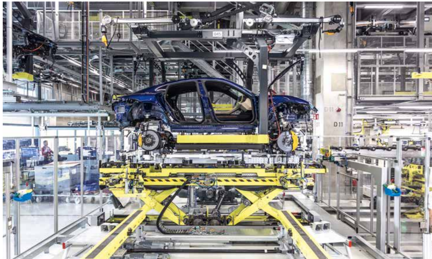
MATRIMONY IN TAYCAN ASSEMBLY: ELECTRIC DRIVE AND BODY ARE JOINED TOGETHER
