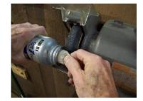
Note: I would recommend grinding the diameter to the same diameter as the rounded and raised ring that is on all pumps which enables the hose to seal tight. See the next paragraph on this.
