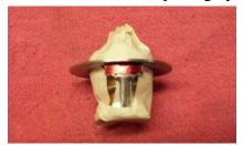
soon discovered that the made in USA Stant seemed to have metal as hard as tool steel: much too tough to snip or file by hand. Although it may not have been necessary, I taped the stat up to keep grit off the internals before I headed for the grinder. It was a blessing in disguise. The tape provided a perfect snug fit as I slid the stat into an old Bayer plastic pill
