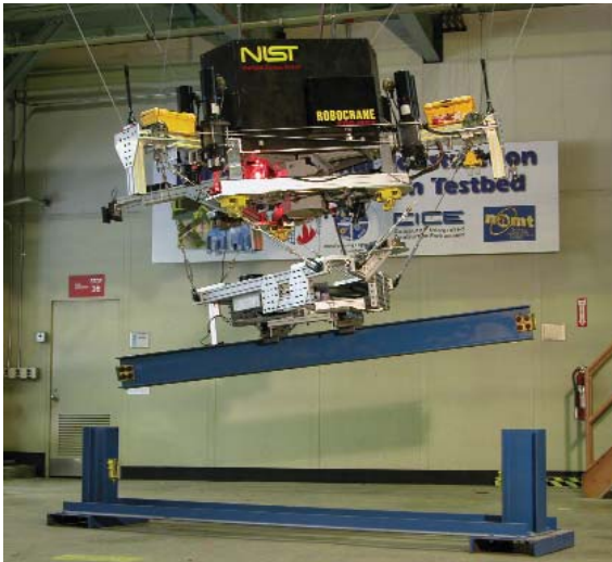
Autonomous steel beam docking using the NIST RoboCrane™.
