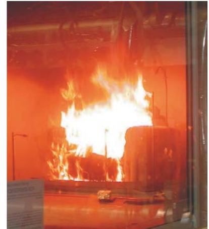
Typical fire experiment used to test the SDFM
