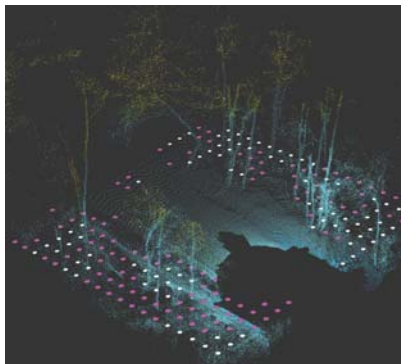
Point cloud of a 20 m x 20 m area showing the identification of trees and bushes.
