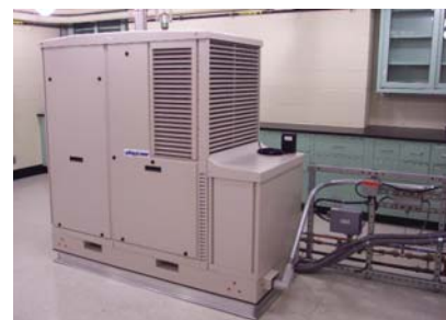
Residential fuel cell undergoing testing in a NIST laboratory.
