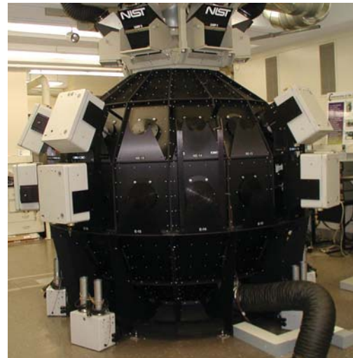
The NIST SPHERE (Simulated Photodegradation via High Energy Radiant Exposure).
