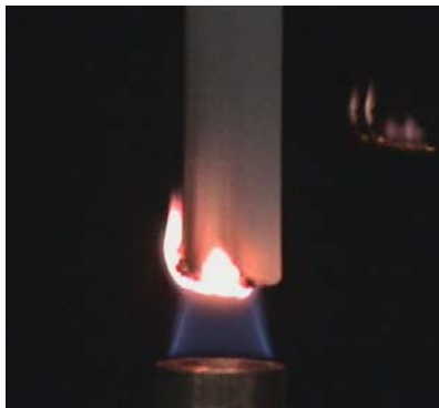
Bench-scale UL94 flammability test.
