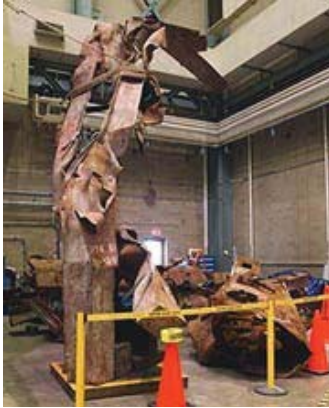
Steel column recovered from site of direct aircraft impact on World Trade Center north tower (WTC 1).
