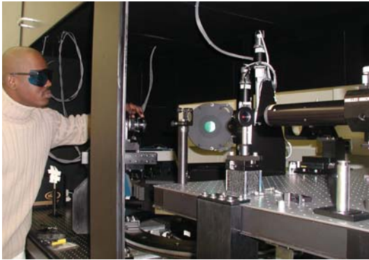
Mr. Joan Jasmin adjusting the two-dimensional detector of the new custom-designed light scattering instrument for measuring the optical properties and microstructure of a polymeric coating.
