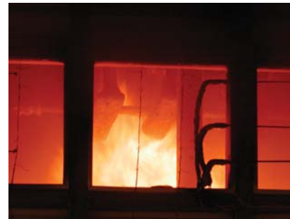
View of fire compartment from air exhaust outlet several minutes after the start of a fire test. Note the flame impingement on the steel trusses and bar
