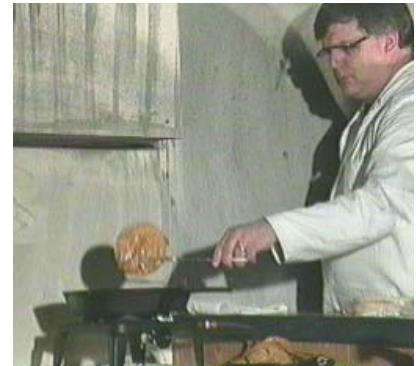
Thomas Cleary deep frying corn tortillas on a gas hotplate produced alarms in ionization alarms only.
