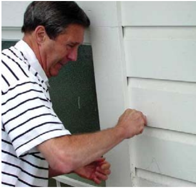
Dr. Walter J. Rossiter sampling a residential house for lead in paint.
