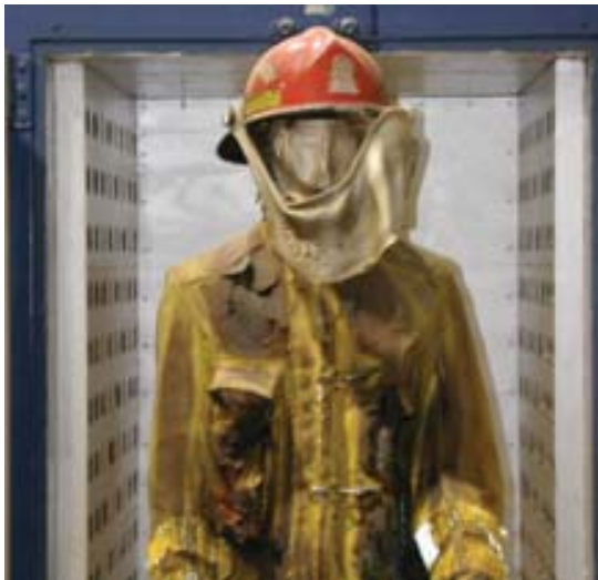
Firefighter protective clothing extreme exposure experiment.
