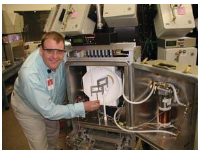
Dr. Christopher White is shown working on custom designed, state-of-the-art, laboratory, sealant testing chambers attached to NIST's SPHERE. Temperature, humidity, ultraviolet and mechanical load can be independently controlled for eight ASTM C719 sealant specimens.
