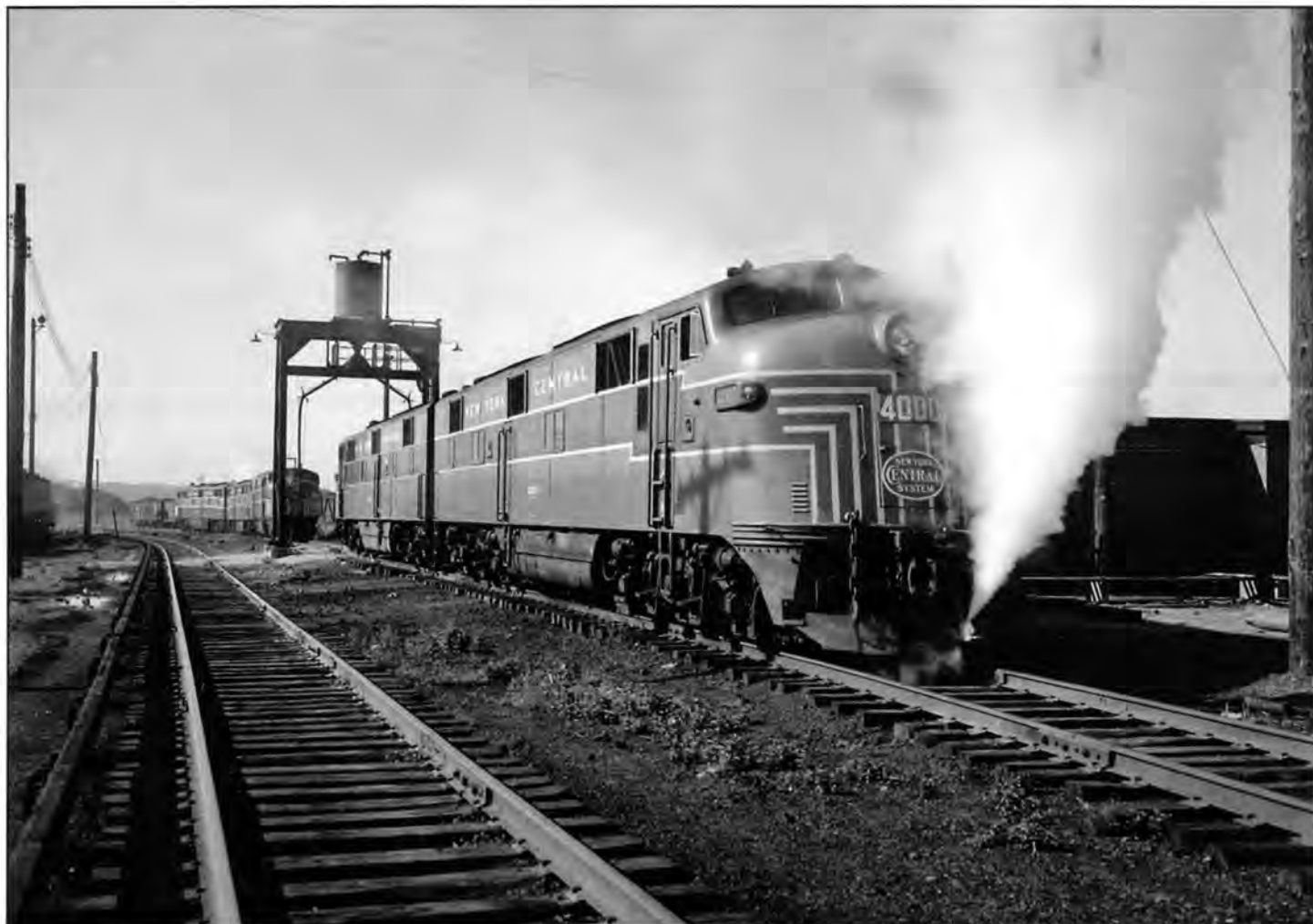
NYC 4000 and a mate pose near the Harmon sand tower on June 26, 1947. Note the consist of reversed grey E7's in the distance, and the electric motor at the extreme left. The coupler cover is open, and the unit is equipped with safety chains and hooks, possibly indicating that the 4000 will be the trailing unit on an outbound train this day. Negative 7758-2.
