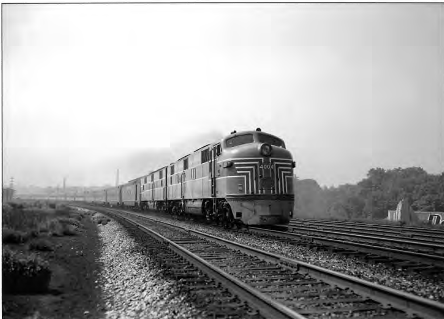
E7 4004 and an unidentified "B" unit are assigned to the Empire State Express on June 27, 1947. A replacement nose door with revised lettering has been applied. The unit does not have safety chains and hooks but does have holes for their application, suggesting that they were portable and applied to trailing units when they were dispatched. Negative 7783-2.
