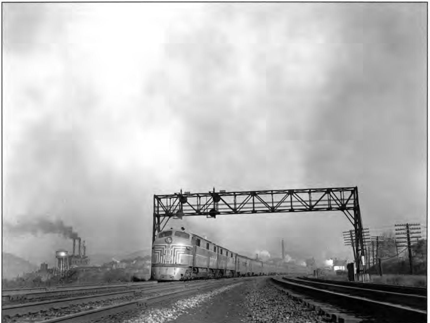
E7 4004 and an unidentified "B" unit have #26's sixteen lightweight cars well in hand on this October day in 1946. The photo demonstrates that two E7's could maintain the schedule of this train with as many as sixteen cars. Negative 7489-1.
