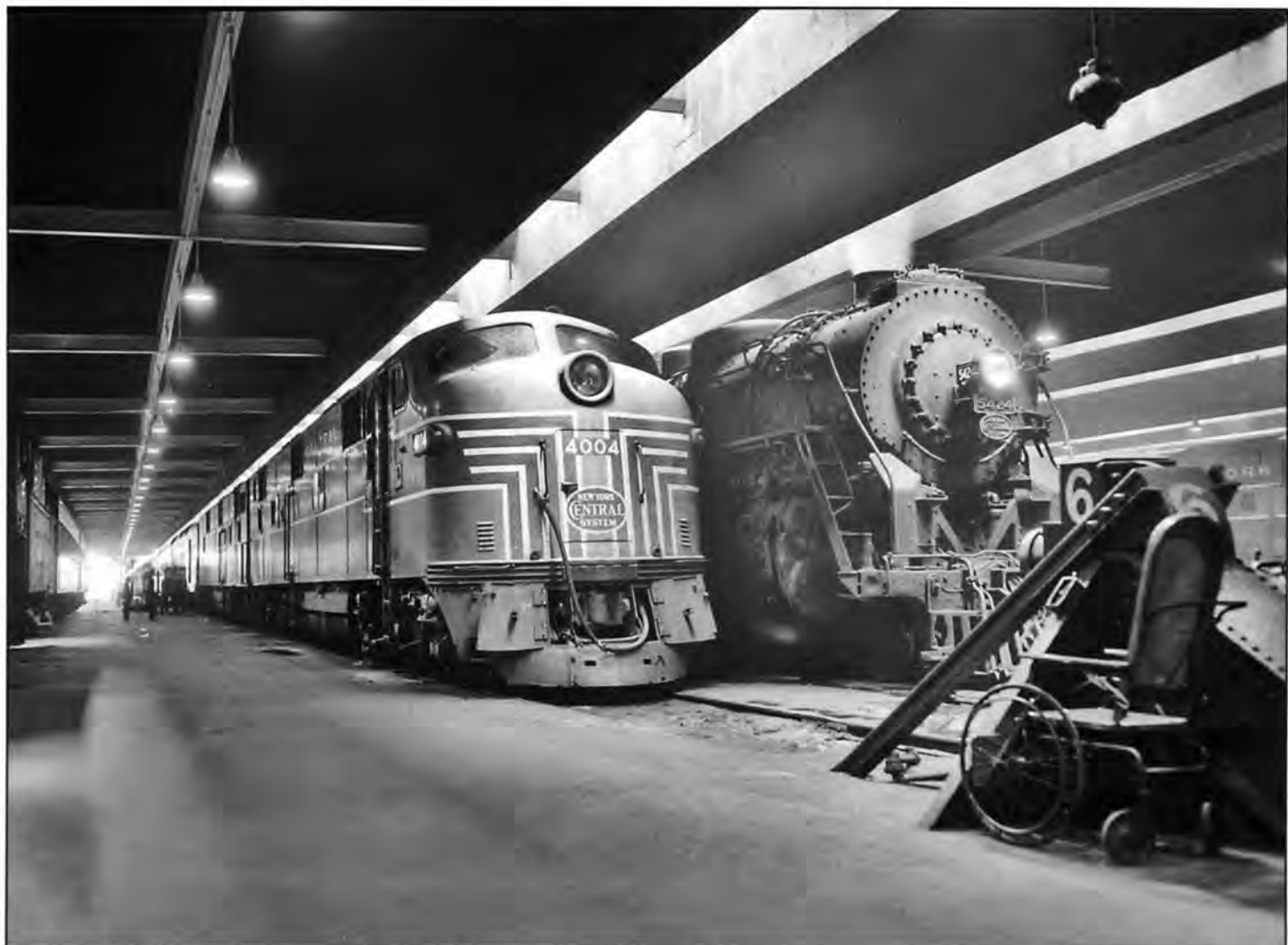
This photo of the 4004 and J-3a Hudson 5424 at La Salle Street Station in Chicago provides a good size comparison between these two high-speed passenger designs. The 4004 has arrived on Train #1, The Pacemaker , on August 24, 1949. Notice the open double coupler cover doors on the diesel. Negative 8664.
