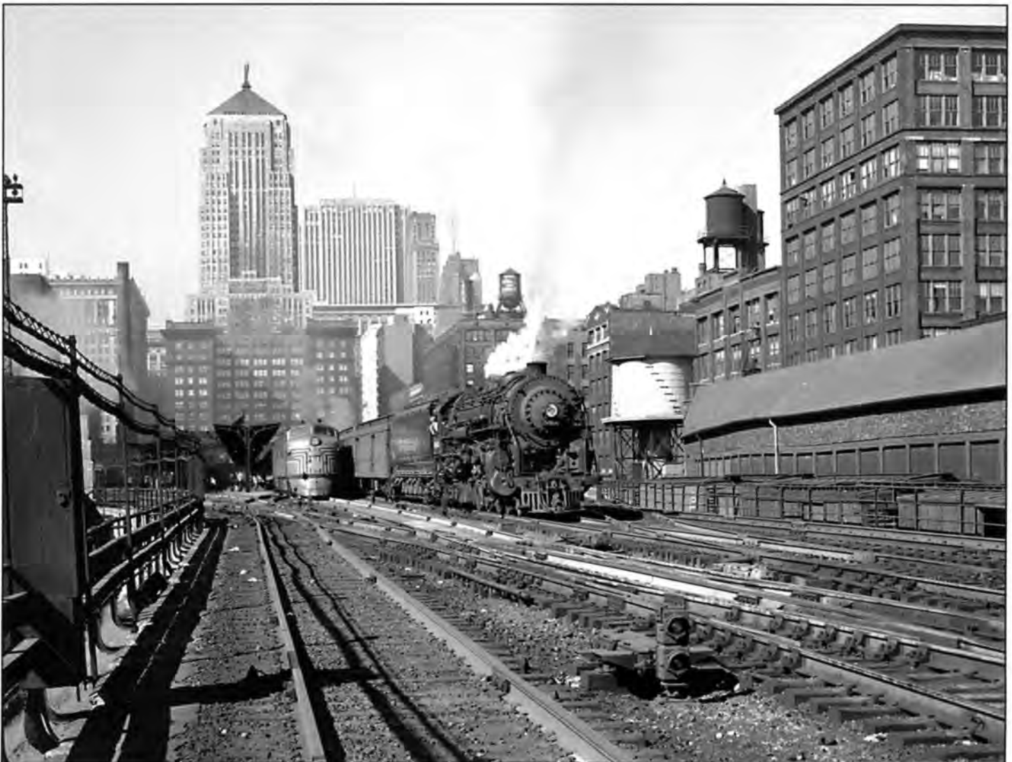
J-1c Hudson 5263 is backing down to its train as E7's, tied to the Century , idle. Lima's PT tender on the 5263 looks almost new. Negative 6989-2.
