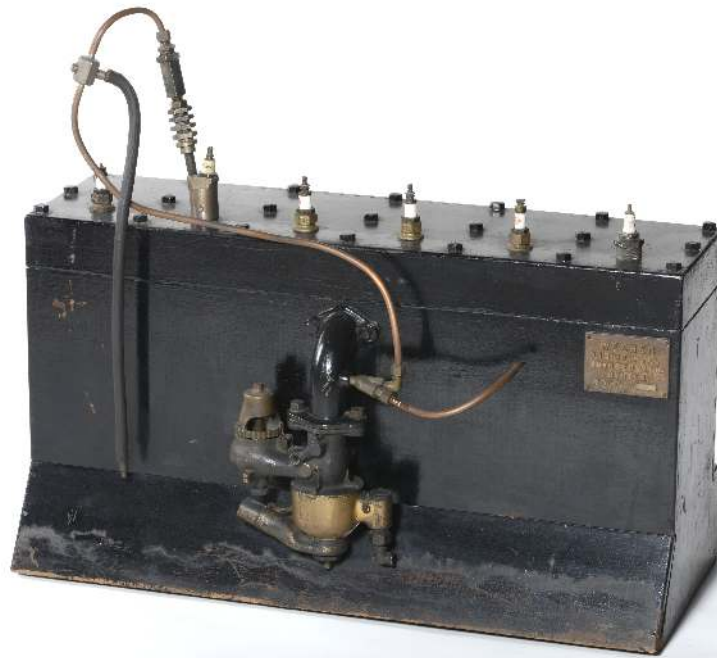
Figure 16.5: This wooden model of an engine was used to display the pieces of a later fuel transforming system, apparently the version using a two-way valve. The device is marked “Weeber Liquid Fuel Transforming System.” NYSM Collection, H-1933.6.2.
