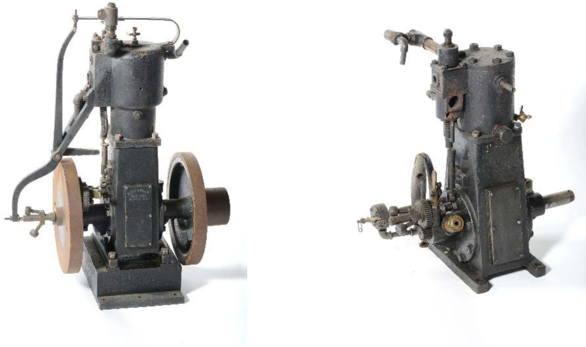
Figure 4.3: Two Weeber stationary engines survive in the New York State Museum. The absence of a carburetor indicates the example ran on piped gas received from a central supply. NYSM Collection, H-1933.6.120 and H-1933.6.6.
