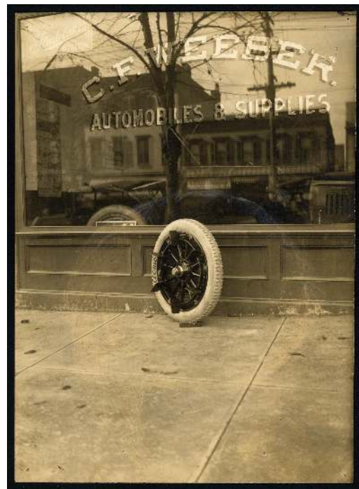
Figure 16.2: Photograph of wheel fitted with a traction ring for publicity purposes leaning against the show window of the C. F. Weeber Manufacturing Works at 170 Central Avenue in Albany. NYSM Collection, H-1987.39.10.
