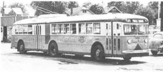
In 1939, the Twin Coach Company built this semi-articulated trolley bus, which bent in the vertical direction only (photograph courtesy of Flxible).
