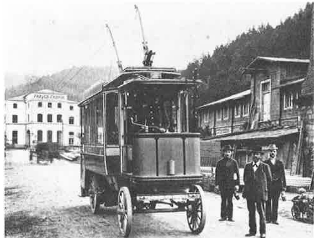
Possibly the first trolley bus that went into revenue service anywhere was in Königstein-Bad Königsbrunn, Germany in 1901 (photograph courtesy of Siemens Company).
