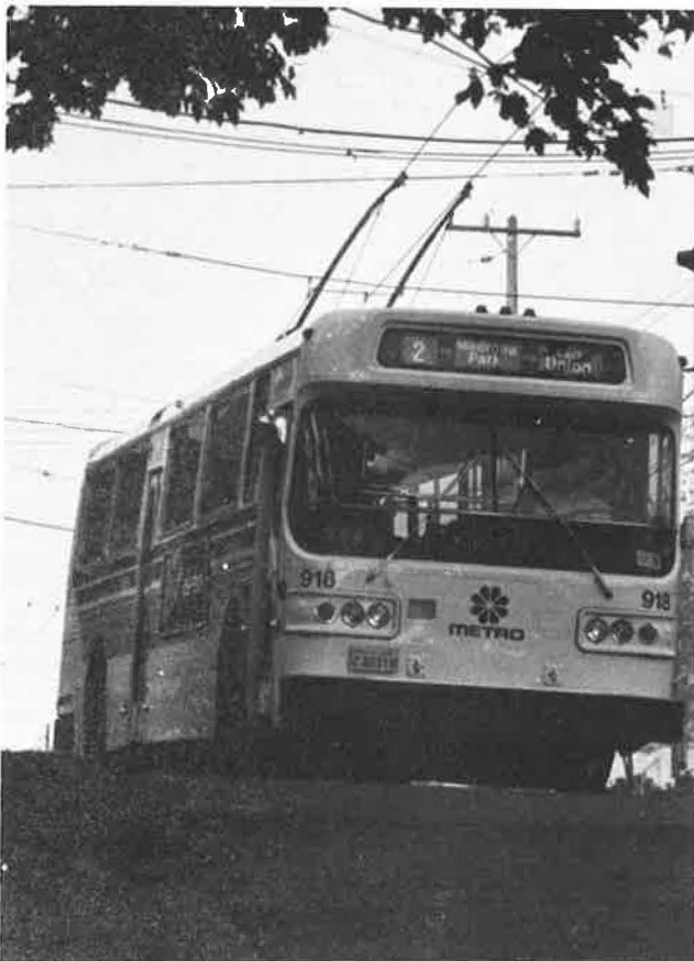
With its poles locked down and the gasoline engine turning its generator, an All-Service Vehicle drives away from the overhead wires (photograph courtesy of NJ Transit).
