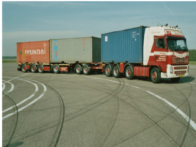
Figure 2.3 An LHV during a swept path test [21]
