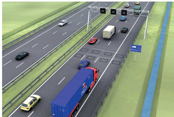
Figure 4.2 Overview Weigh-In-Motion Video system (source: Directorate General for Public Works and Water Management, 2004)
