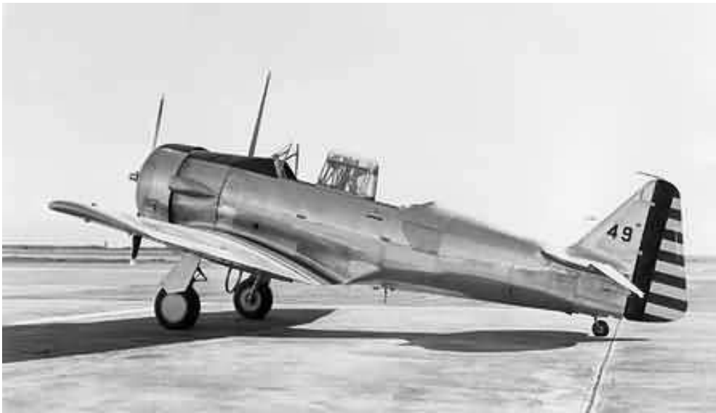
BC-1A. Photo circa 1941. This is a USAAC aeroplane based at Oakland, California with a trainer unit number. The fuselage is natural metal with a clear top coat and the top and bottom of the wings are Orange Yellow. The rudder bears the single Insignia Blue vertical and thirteen Insignia Red and Insignia white alternating horizontal stripes which appeared from time-to-time on the rudders of various USAAC+ and USN/USMC aircraft from 1926 - 42. Note the retractable undercarriage, triangular rudder and metal panels on the fuselage. This aeroplane is just a hair's width from AT-6 and is visually distinguishable from it only by the large D/F loop under the forward fuselage (or is it ? - see below).
