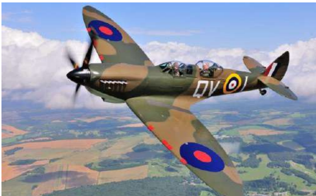
Two-seat Spitfire Mk. IX. The instructor sits behind and slightly above the student up front. This arrangement wreaked havoc with the Spitfire IX’s center of gravity moving it far aft causing the usual concurrent instability at lower airspeeds. Accordingly, intentional stalls and spins were prohibited.
