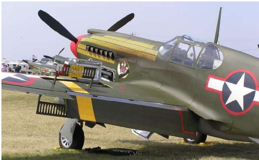
Restored North American A-36 "Apache" fighter-bomber. Note the speed/dive brakes on the upper and lower surface of the wing that were unique to this variant. The immediate predecessor to the P-51, "Apache's" Allison engine was un-supercharged and therefore the aeroplane could not adequately perform above 15,000 feet. However, upon a complete re-design and the installation of a supercharged Rolls-Royce "Merlin" engine, the same engine installed in the "Spitfire" and "Hurricane", the P-51 was transformed into what many consider to be the finest fighter of WWII. The insignia on this aeroplane is the short-lived, red-outlined stars and bars, which appeared only from 28 June 1942 - 14 September 1943.
