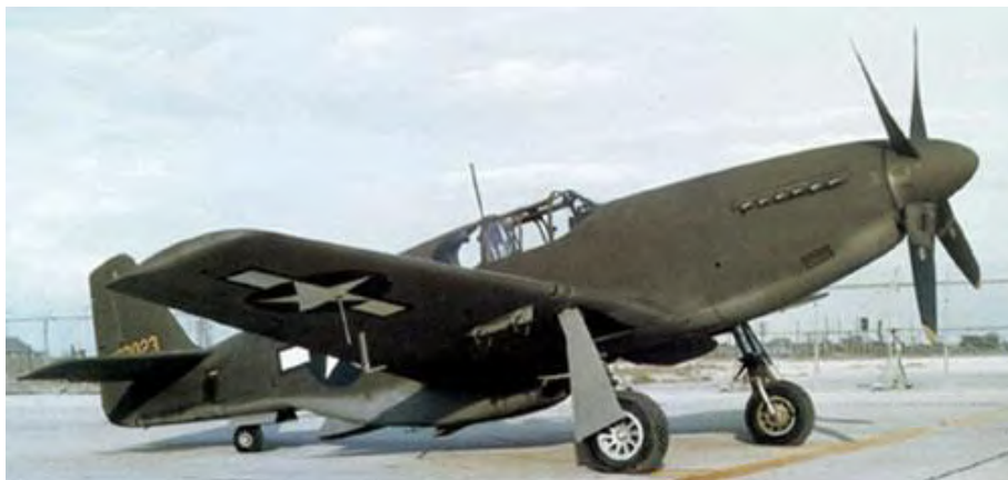
P-51B. This was the earliest "Mustang" to see combat and was the fastest of all the "Mustang" variants during WWII. The bubble canopy of the "D" model, whilst granting excellent 360 degrees visibility, created a good deal of drag as opposed to the more aerodynamically efficient fastback "B" variant. This is a WWII era photograph taken at March Field, Riverside County, California in which the colours are unusually excellent and accurate. This "Mustang" is seen here in "ANA Olive Drab 41" and "ANA Neutral Grey".
