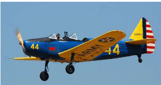
Beautifully restored PT-19A Primary trainer in "Orange/Yellow" (FS13558) and "True Blue" (FS 15102).
