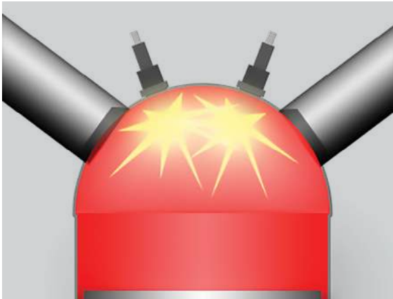
The air and fuel are compressed by the piston, then the ignition system adds the spark to create a controlled explosion.
