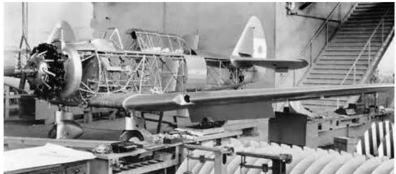
NA-18 showing steel tubular under-structure with the aluminium panels removed for maintenance.
