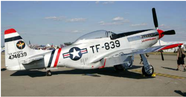
Korean War era TF-51D, two- seat Mustang. These can be easily distinguished from single seat F-51Ds by the elongated, raised bubble canopy to give the rear-seater a little headroom.
