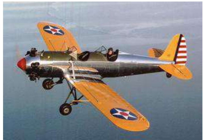
Ryan PT-22 in mid- WWII “bare metal” and “ANA Orange Yellow”. What is commonly called “bare metal” was, as seen here, actually the unpainted aluminium skin coated with a clear top coat to protect it. Many of the so-called “bare metal” finishes were actually aluminium-coloured paint with a clear top coat. A decent clear top coat was a necessity for aircraft that were to spend much of their time parked outdoors in the weather as well as all aircraft carrier- based aeroplanes.
