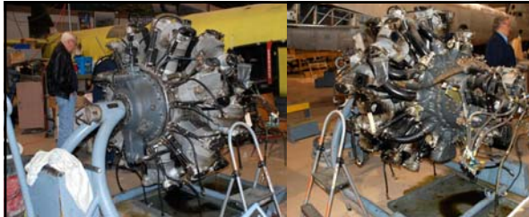
Above: the R-2600 Wright Cyclone series engine was introduced in 1939, initially rated at 1,500 hp. With improvements, it later reached a rating of 1,800 hp. In military use, it was used on U.S. Army Air Force A-20s, A-24s and B-25s as well as some U.S. Navy torpedo and patrol bombers. It gained fame powering the Boeing Model 314 "Clipper" flying boats. It held fourteen cylinders in two rows in an air-cooled radial configuration. Maximum horsepower and rpm was 1,700 and 2,600 respectively. It weighed 1,980 lbs. and cost $16,500. After the end of WWII, the R-2600 was superseded by larger radial engines.
