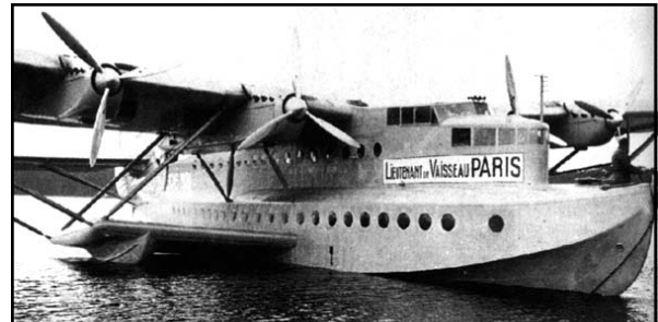
“...The French had a try, too, at producing the ‘world’s largest’ flying boat. It made its bow on Jan. 15, 1935. With the Do-X no longer in the running, the French entry in the transoceanic sweepstakes seemed to deserve the title, even at a somewhat lower gross weight, 37 tons. Its name – Lieutenant de Vaisseau Paris – was in keeping with its size. Its wingspan was 162 feet. Its double-decked hull, 30 feet high, was 104 feet long. Its six engines, with four tractor and two pusher propellers, produced 5,100 hp...” 496 Popular Science , June 1963
