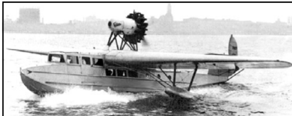
"...latest of Fokker creations is this graceful flying boat with cabin for eight passengers. Driven by a 550-horsepower engine, with 'pusher' propeller above wings, it is designed for a speed of 125 miles an hour. A kitchen and sleeping quarters permit week-end trips or long cruises in comfort..."
