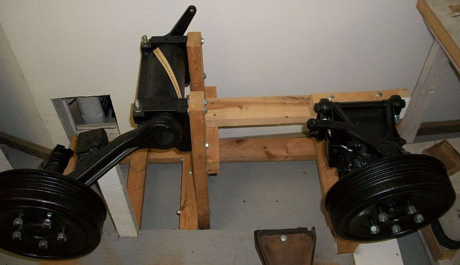
Above: caption: “Tucker rear suspension rubber torsion tube (left) and sandwich-type front suspension (right) - used on car Nos. 1001–1025”
