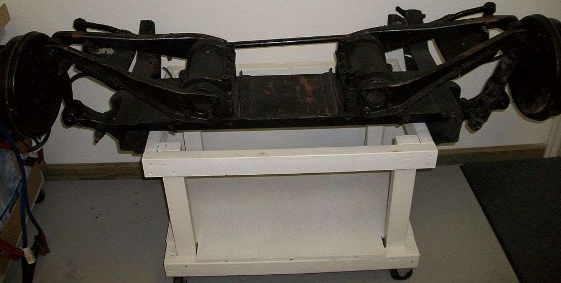
Above: caption: “Tucker Rubber Torsion Tube (version No. 2) - front suspension used on car Nos. 1026 on. This unit taken from car No. 1046 for V8 conversion.”
