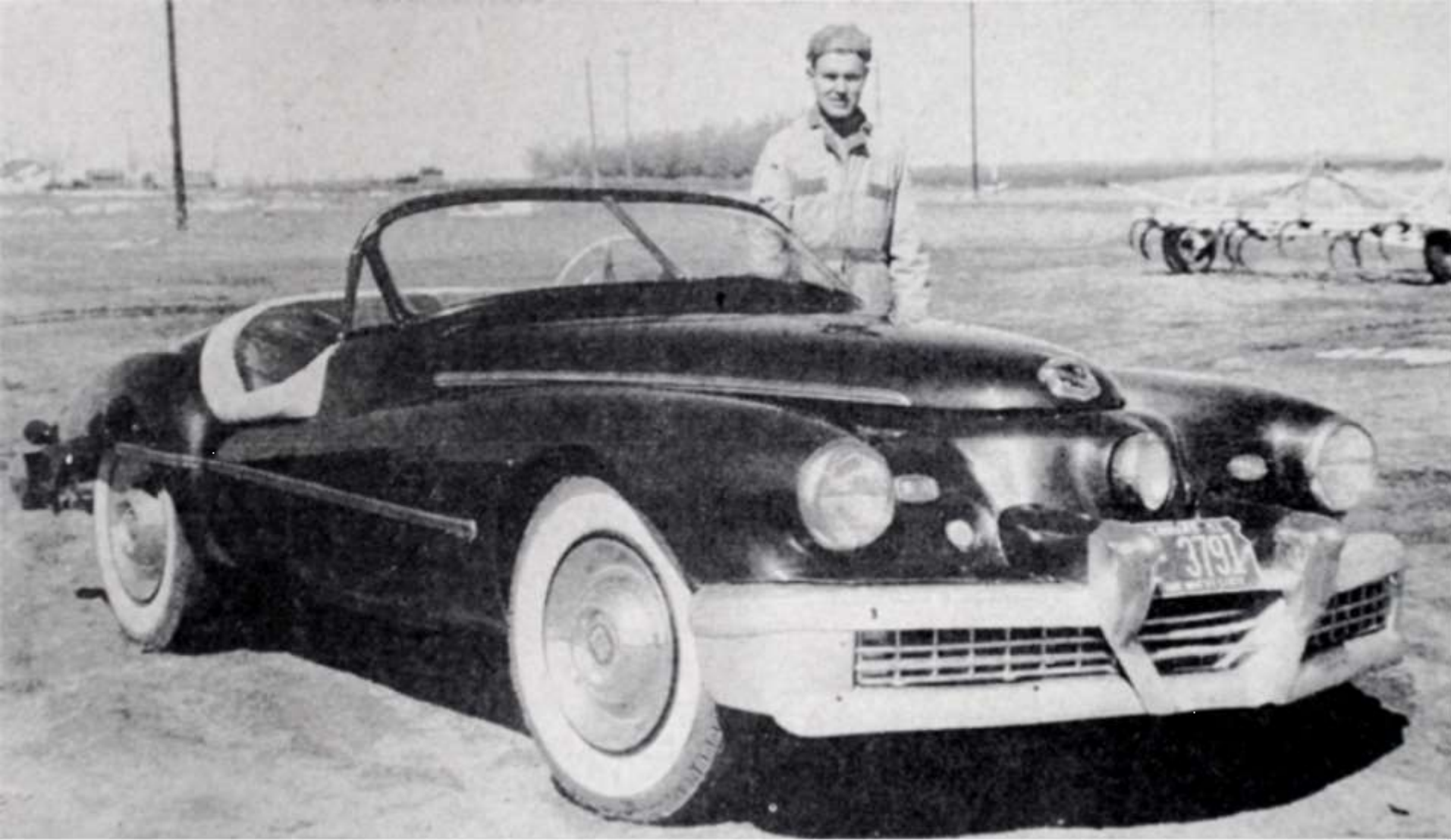
Above: George Esch built a fiberglass Tucker Convertible replica (completed in 1997). The car was based on a 1966 Chevrolet Corvair. He calls it the “Glass Goose.”
