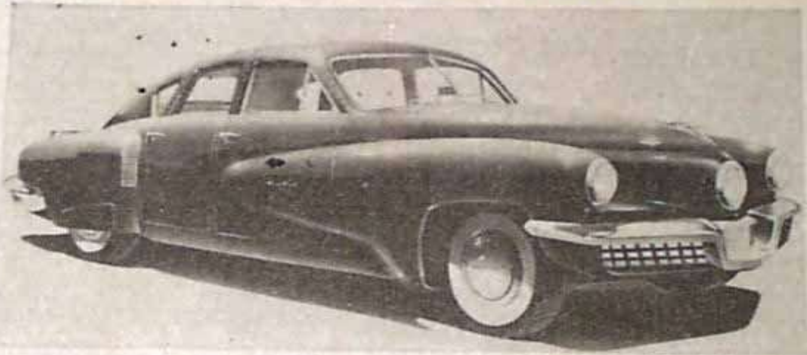
THIS IS THE PILOT MODEL OF THE TUCKER 48 Unusual design features rear engine
