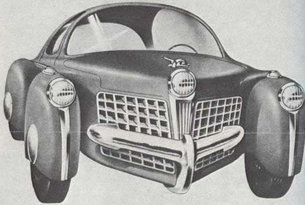
LONG, LOW, and streamlined, the Tucker Torpedo has doors that extend into the top for easier getting in and out. Brakes are of an automatically adjusting type developed originally for racing cars. A new engine can be installed in 15 minutes when necessary.
