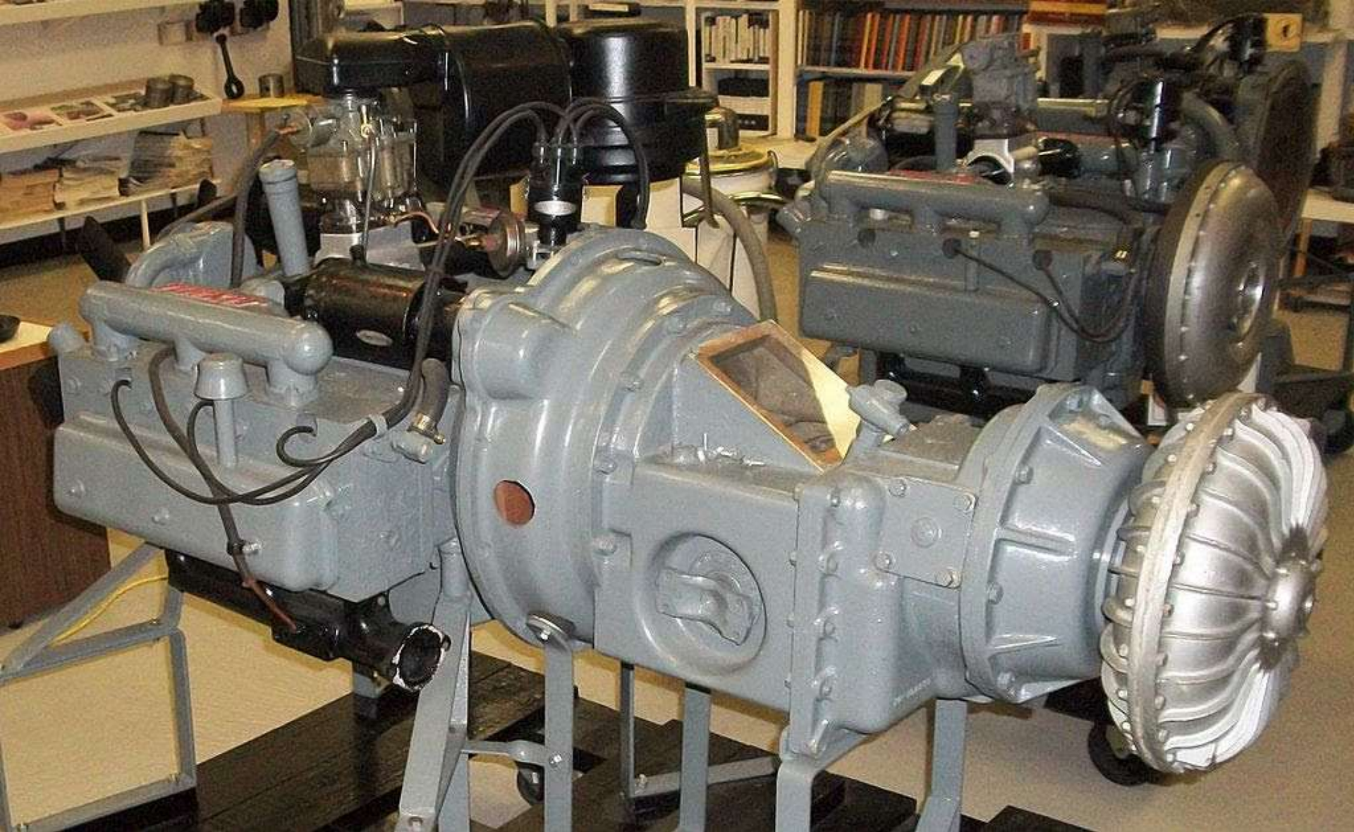
Above: caption: “R-1-2 transmission (recovered from car No. 1042; note second torque converter on the end)”
