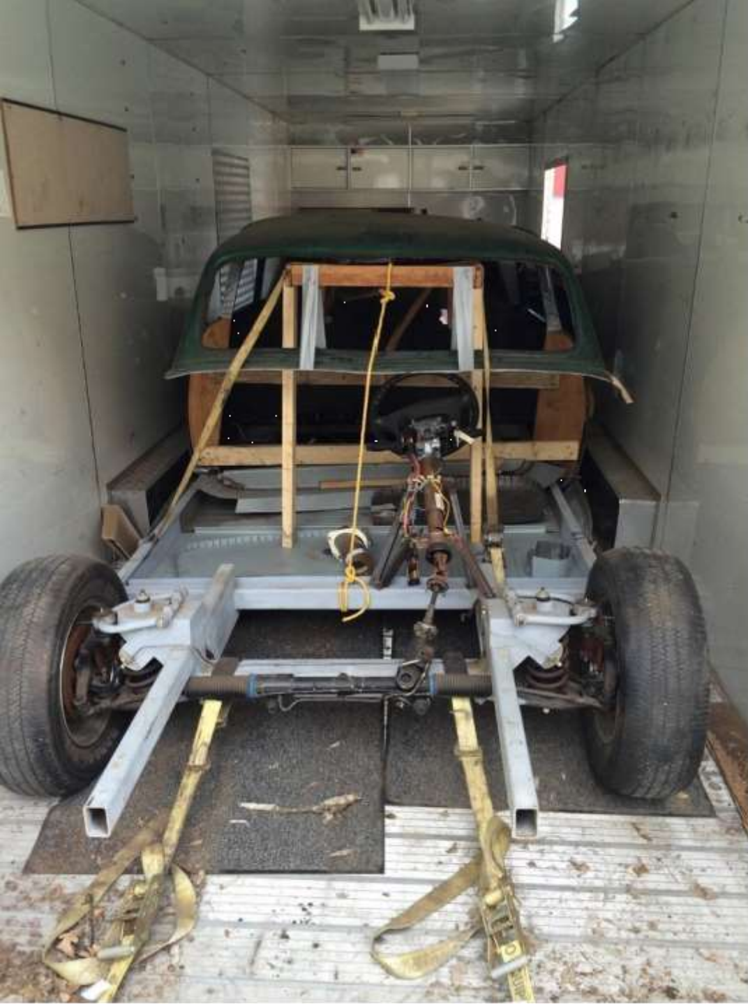
Above & Left: one of four fiberglass replica Tuckers built for use in the Tucker movie. This movie Tucker was built for the scene whereby car No. 1027 rolls over at the Indianapolis Motor Speedway while participating in a 24-hour endurance test.
