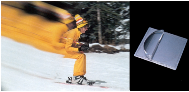
Figure 48: A special filter (on the right) permits the simulation of motion blur (from [Kod81]).
