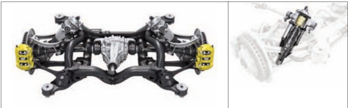
Fig. 75: Rear axle and air spring strut on rear axle with Porsche Active Suspension Management (PASM)
