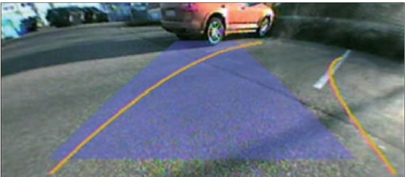
Fig. 127: Image output of reversing camera with dynamic guide lines
