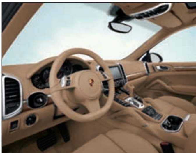
Fig. 63: Steering wheel with 2 sliding buttons in the Cayenne Diesel (not for US) in Luxor Beige
