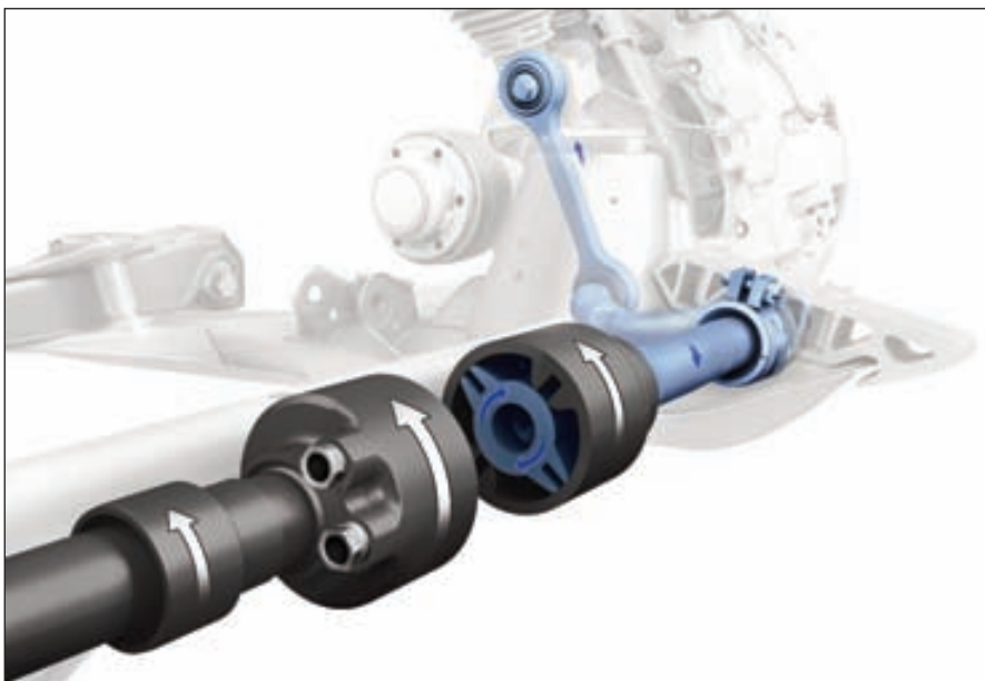
Fig. 77: Functional representation of active anti-roll bar (PDCC)
