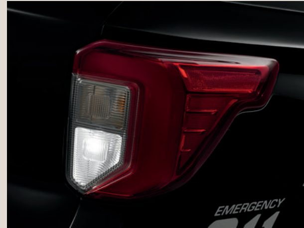
Taillamp Lighting Solution (66B). Includes halogen base lamps, plus (2) integrated hemispheric lighthouse LED side warning lights.
