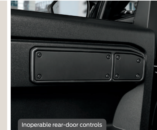
Inoperable rear-door controls
