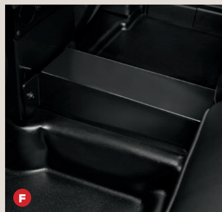
Rear console plate. Interfaces with front console mounting plate and extends through 2nd-row occupant area to seat bottom (acting as wiring conduit on top of transmission tunnel).
