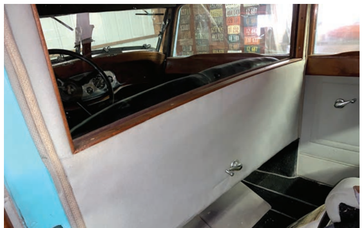
Shown are the unique features of this 1931 Berline, a 1932 style dash and a division window
