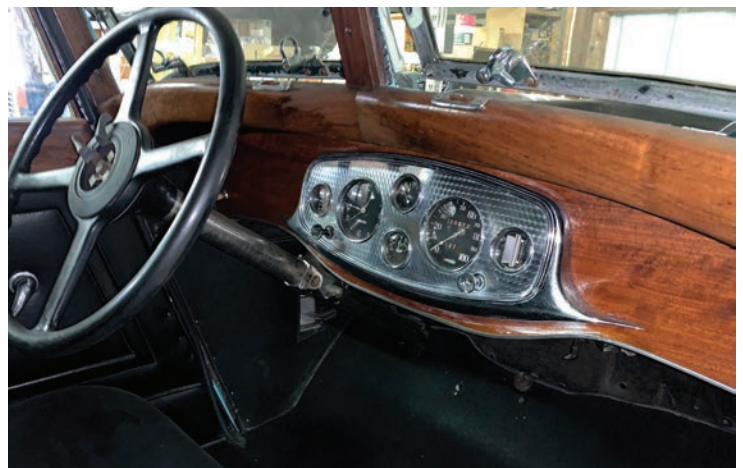
Shown are the unique features of this 1931 Berline, a 1932 style dash and a division window
