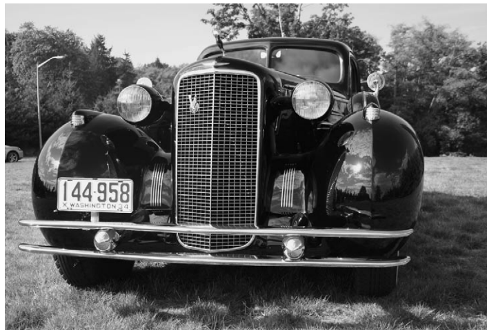
The iconic Cadillac grille and energy-absorbing "bi-plane" bumper enhance the distinctive styling of the Coupe
