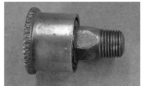
6. Reassembled grease cup. "O" ring is not visible once installed.
