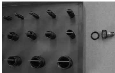
3. Select "O" ring of workable I.D. and O.D. "O" ring needs to be tight enough so it doesn't rotate in groove. O.D. of "O" ring must allow cup threads to pass without being too loose or too tight. If necessary, you could grind/sand away a bit of "extra" O.D.
