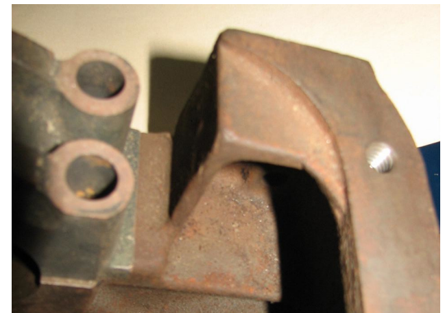
Here is what the drivers side on the Oakland block looks like. No allowance is made for the shaft to be located here.
