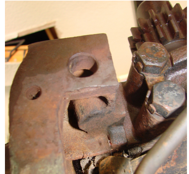
This is what the 1932 Pontiac block looks like on the passenger side. This would have been drilled out on an Oakland 1930/31 block.
