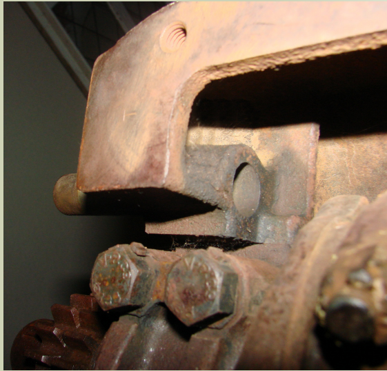
Here is the drivers side on the Pontiac block where the shaft is installed. You can see how different this is from the Oakland block.
