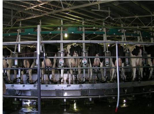
80 stand rotary, computerized milking parlor. (2009) 122
