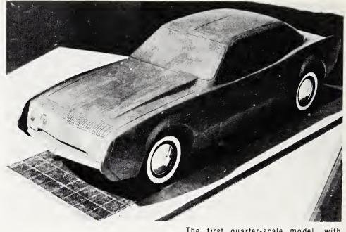
The first quarter-scale model, with superstructure firmed up. Gene Hardig later said upper grillework was unnecessary.
