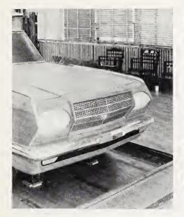
Halogen or glass-covered head lamps figured in 1964 plans, but ultimately conventional sealed beam lamps were fitted.
