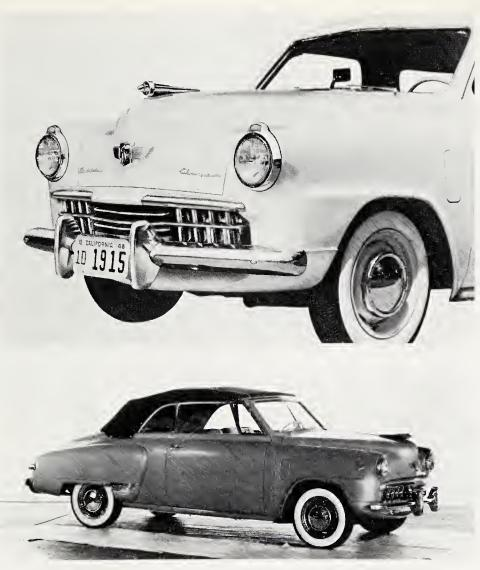
Airbrushed photo of 1948 Champion front quarters displays curved one-piece windshield—and revised '48 grille. The one-piece windshield was used from 1947 to 1950 only on five-passenger coupes, Land Cruisers and convertibles. Other models had flat two-piece windshields. In 1951 all body styles used curved one-piece glass.
