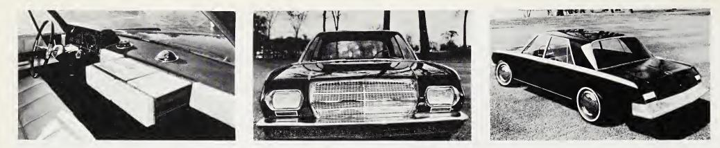
Views of the Stevens' 1965 model. Note raised computer-style instrument panel, 'polo mallet' steering wheel, crash-padded vanity, accessory compass and clock, recessed door handle, interchangeable body parts.
