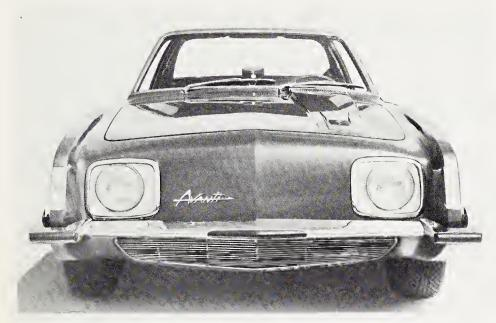
New radiator grille appeared in August 1963 with square-bezel head lamps, but some round-head-lamp models were also fitted with the grille.
