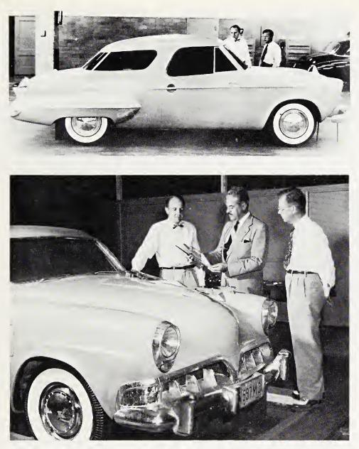
Bourke-Koto study Model N proposal. Different styling ideas include grooved roof, dropped waistline, built-in door handles, pontoon rear fenders. Comparison Chevy lurks in background.
