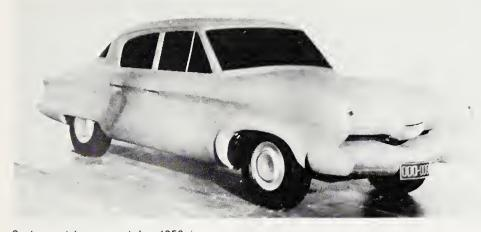
Scale model proposed for 1950 incorporated Loewy spinner, floating wing between fenders. Contoured bumper proved too expensive to produce.
