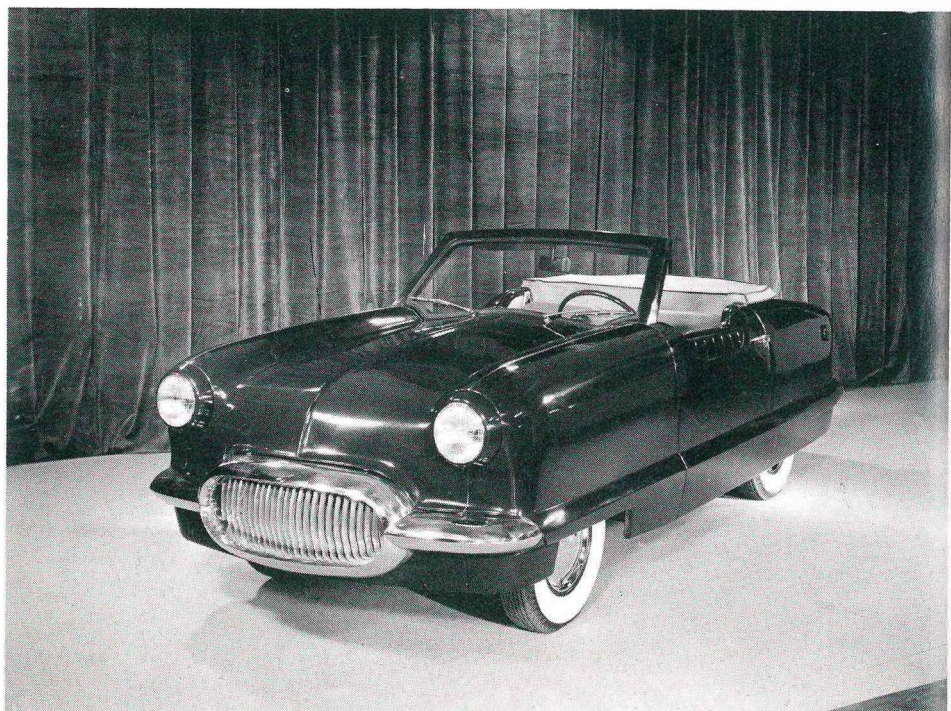
60. Thinking aloud in America: Nash's N.X.I. with FIAT 500 engine, built in 1950 to test customer reactions to a small car.
