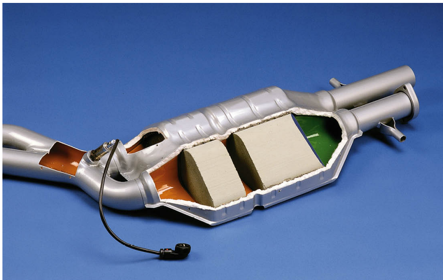
A Mercedes catalytic converter, with the lambda sensor upstream of it, measuring oxygen levels in the exhaust and signalling the engine's ECU to adjust fuel-air mixtures and keep emissions to a minimum.
