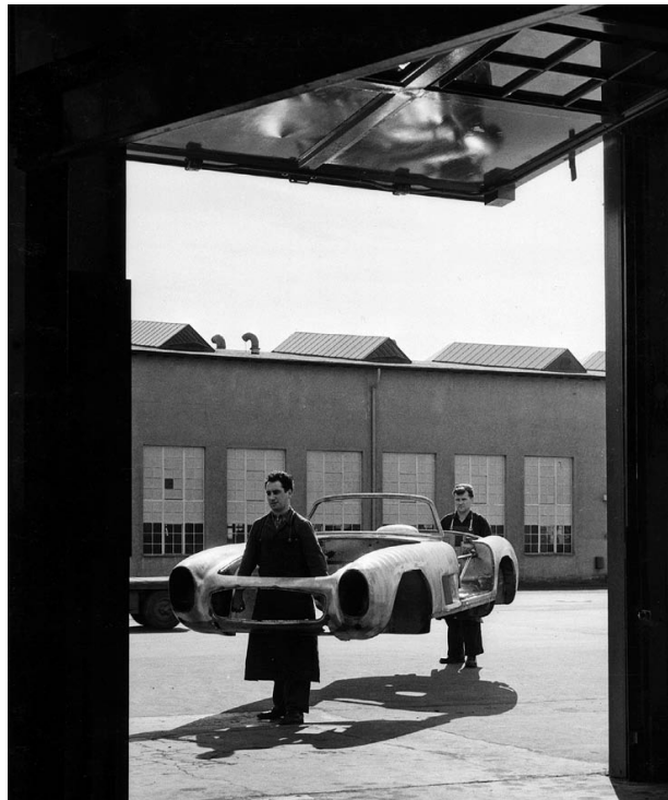
Fascinating picture of the lightweight roadster body being carried to the production line. The untrimmed shell tipped the scales at 185kg (407lb).
