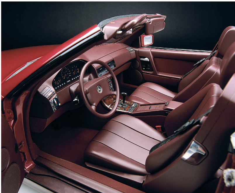
An interior styling mock-up, with numerous components, such as air vents and light switches, represented by printed card stuck in place. Note also the rather characterless seat upholstery, which duly became more luxurious, and the rear compartment arrangement, set up as a 2+2.
