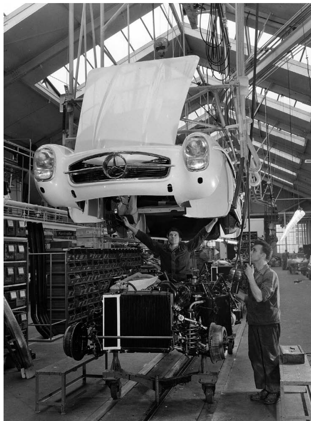
Production shot from 1958, with a 300SL roadster being tended to on the line. Note the modified spaceframe chassis.
