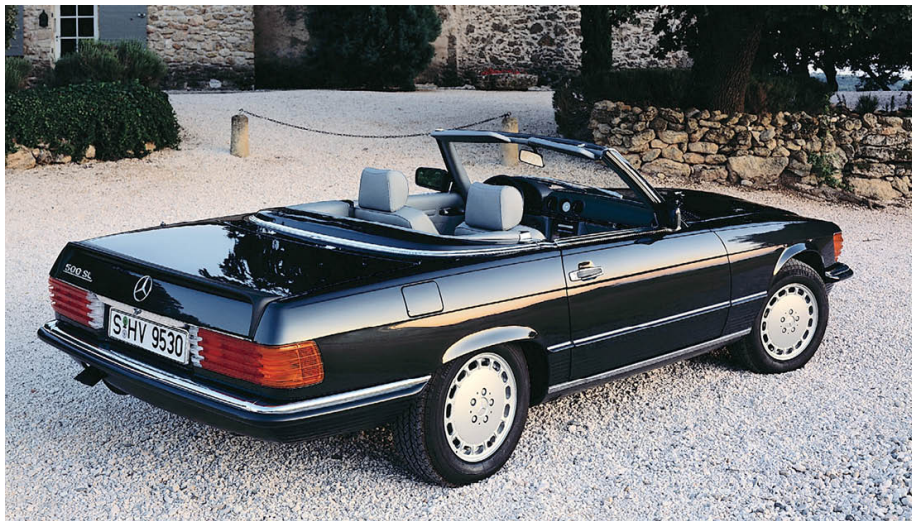
One of the last R107 models, this being a domestic market 500SL, introduced at DM 89,091. Weighing a hefty 1610kg (3540lb), it was still capable of 140mph (224kph) and a 0-60 time of 7.8 seconds. Note the late-style alloy wheels, introduced for the 1986 season. R107 production finally came to an end in July 1989.
