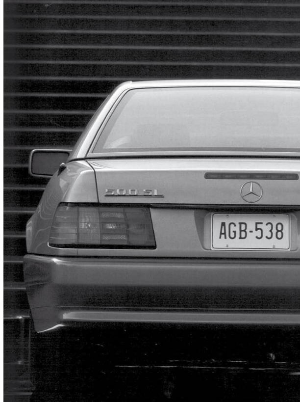
Tail of a US-spec 500SL, with a third brake light worked into the bootlid.
