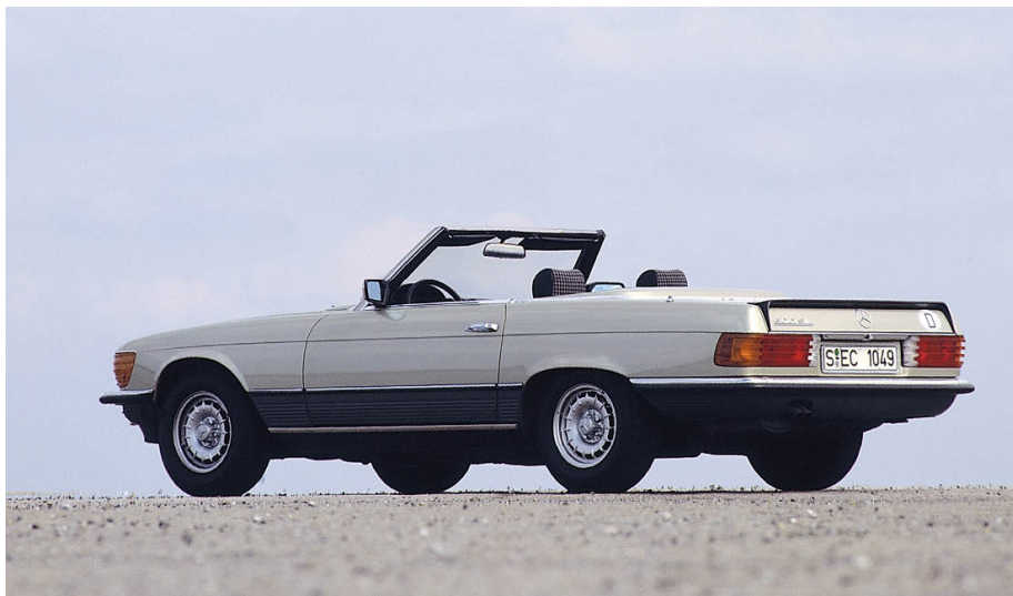
A 1981 Model Year 500SL. Note the dark grey lower section, applied to five-litre cars when finished in certain colours, and the rear spoiler. All cars received an aluminium bonnet at this time.
