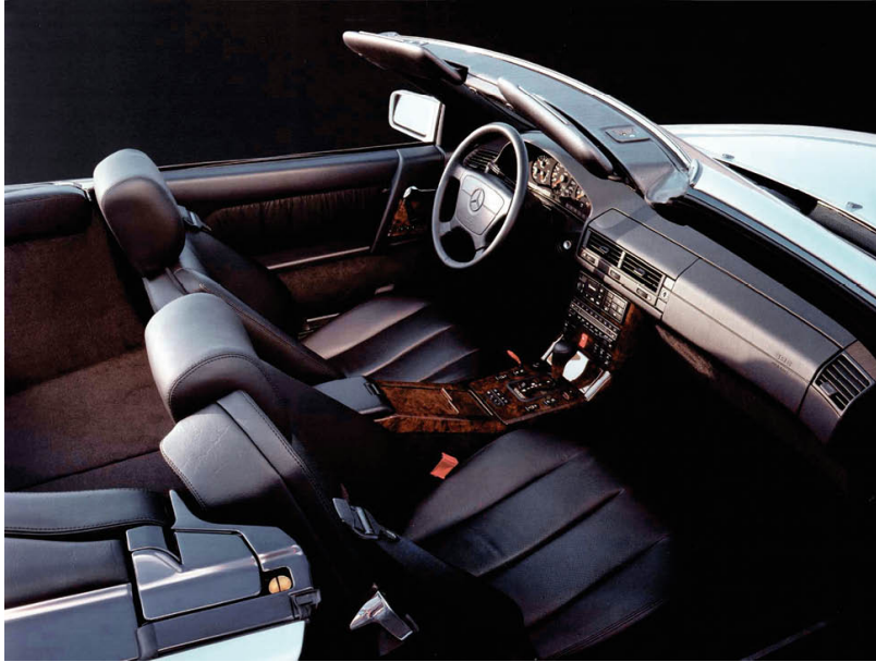
Interior of an early V12 SL. Note the unique gearlever and the extra wood applied to the centre console area, as well as the smaller-diameter 'Sportline' steering wheel introduced in mid-1991.
