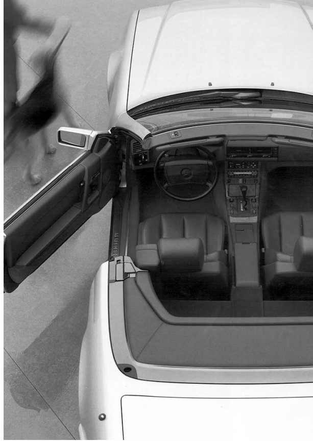
Overhead view of the new SL in North American specification, giving a rare view of the carpeted rear compartment and the stainless steel treadplates.
