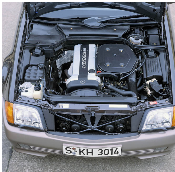
Engine bay of the 300SL-24 model. All six-cylinder SL units were mounted at a 15-degree tilt to lower the bonnet-line.
