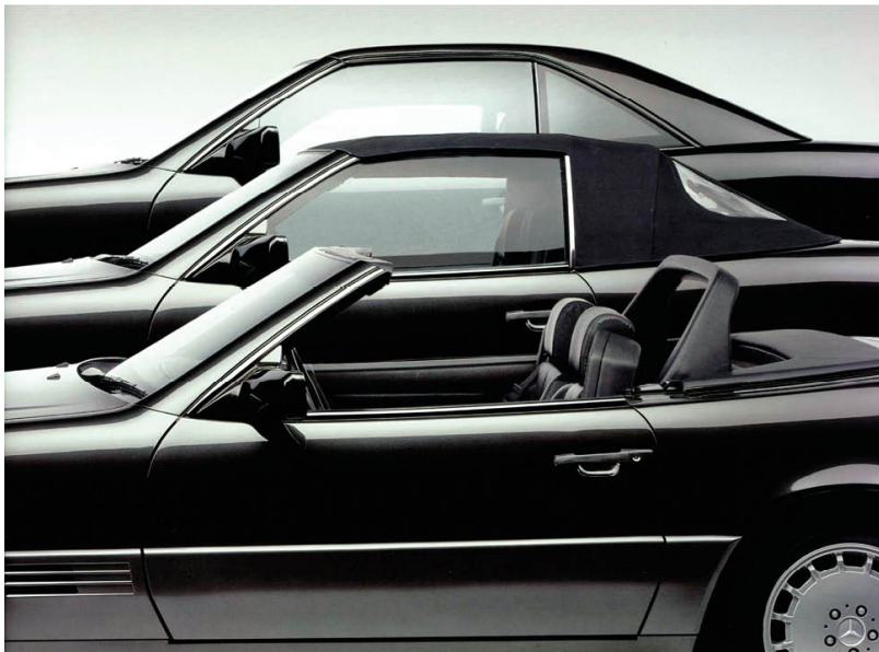
The R129 hardtop in the background, with the soft-top open and closed in the foreground, thus giving an image of the roof profiles.
