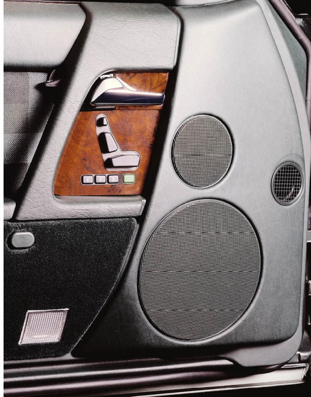
Power seat controls (with memory facility) and audio speakers on the inner door panel.
