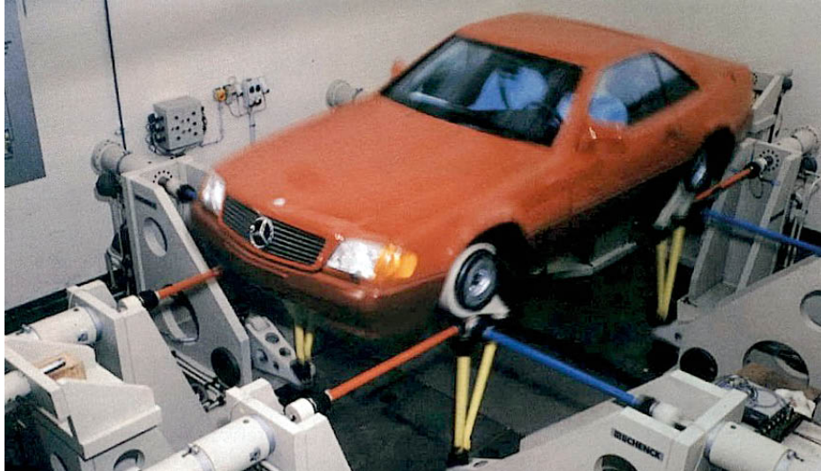
Another prototype on a Schenck shaker rig.
