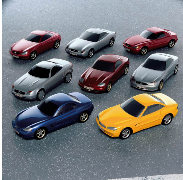
Scale models showing some of the styling proposals for the R170 SLK.
