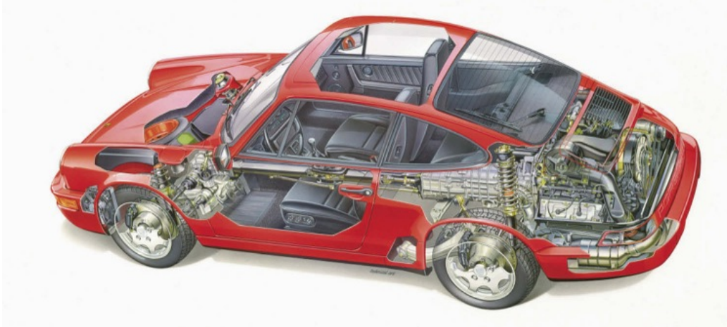
Cutaway drawing of the C4, clearly showing the suspension, brakes, and general layout of the vehicle.
