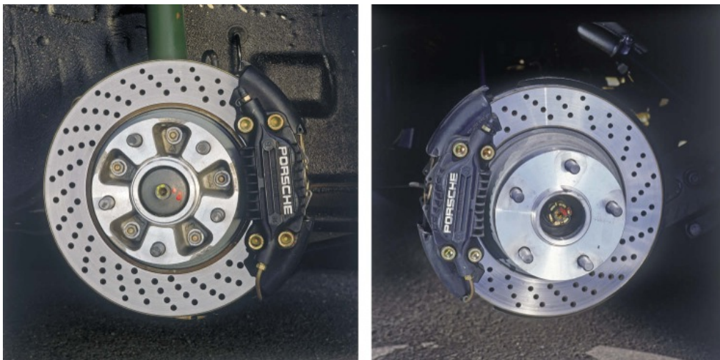
The offside front (above) and rear (above right) brakes of the Turbo. Comparison with the brakes of the NA car (illustrated on page 39) will reveal a number of significant differences between the two systems, not
