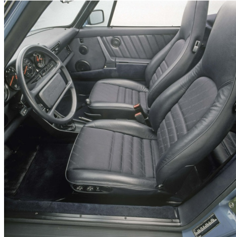
Catalogue picture of the US-spec Carrera for 1988. Note the power seat switches, and the tiny horn symbol added to the steering wheel centre pad on American cars.
