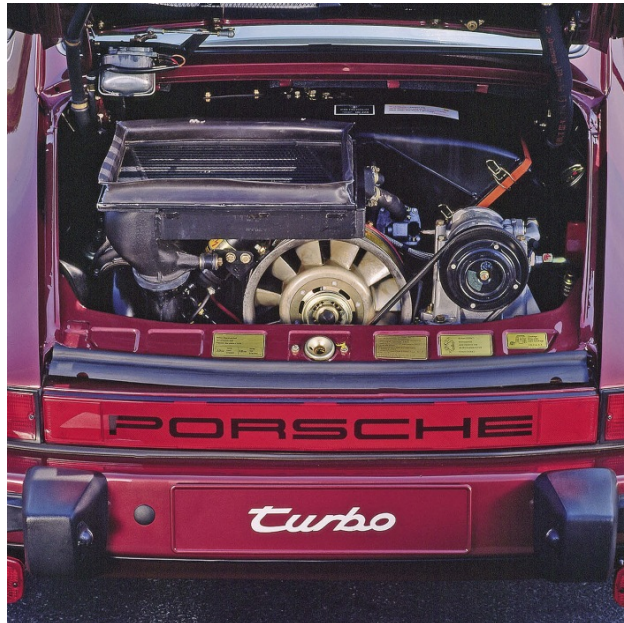
The crowded engine bay of the 3.3 litre Turbo.
