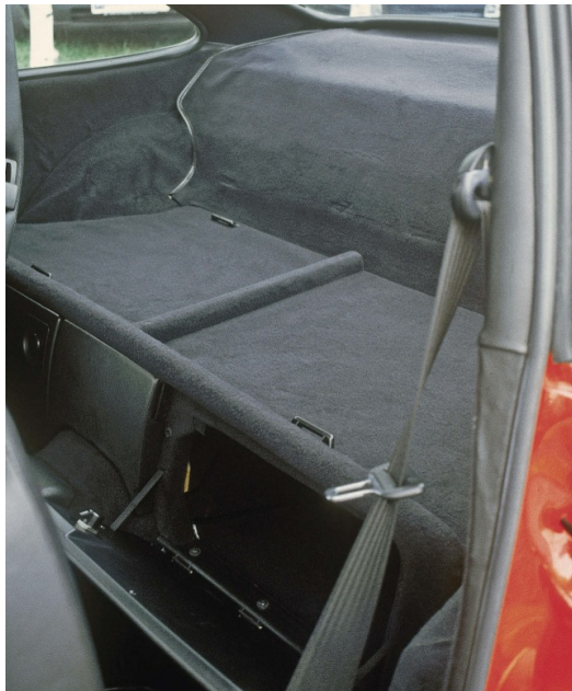
The rear shelf and storage bins that were fitted to the RS America.
