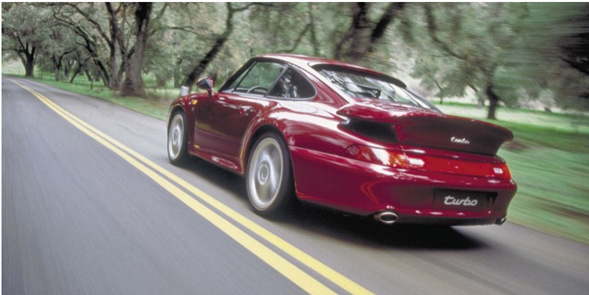
The Turbo at speed. Note the oval tailpipes of the turbocharged car, which had a stainless steel exhaust system.
