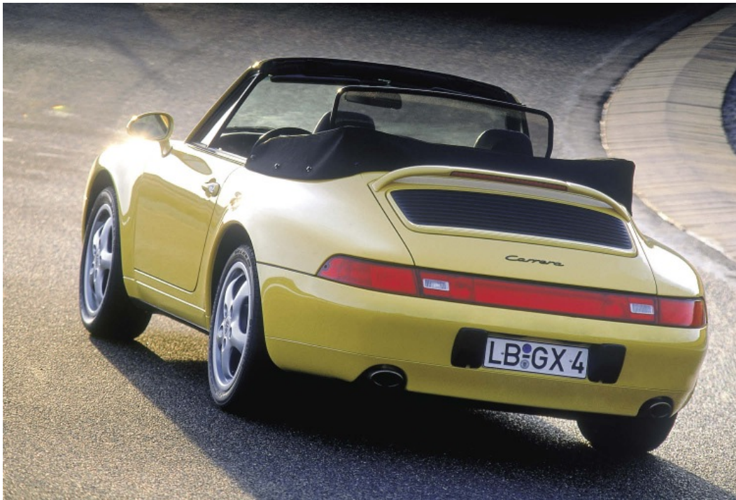
A US cabriolet with windblocker erect. Note the small buffers around the rear number plate on the American-spec cars, and the high-mounted rear brake light in the hoop atop the engine cover.
