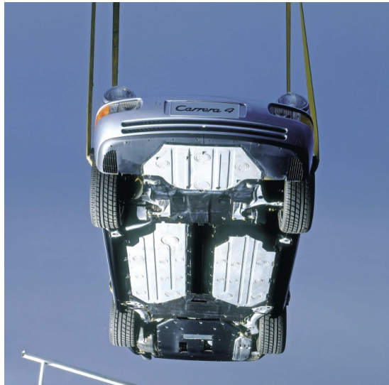
A most unusual photograph of the Carrera 4, but one that clearly shows the amount of detail work on the underbody of the 964 series.
