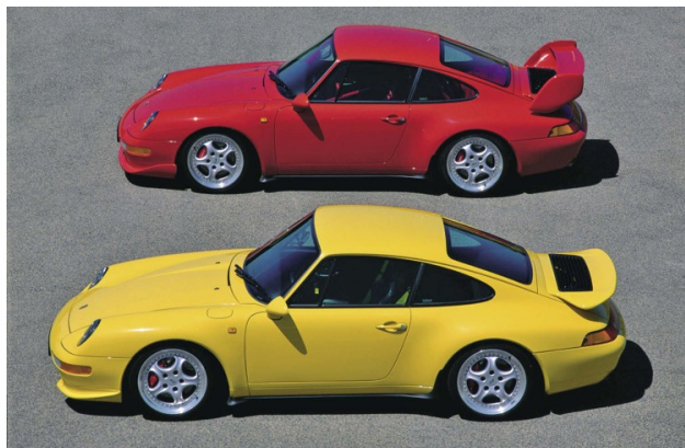
The RS (nearest the camera) and RS Club Sport. The RS sat 30mm (1.2in.) lower than the regular Carrera.
