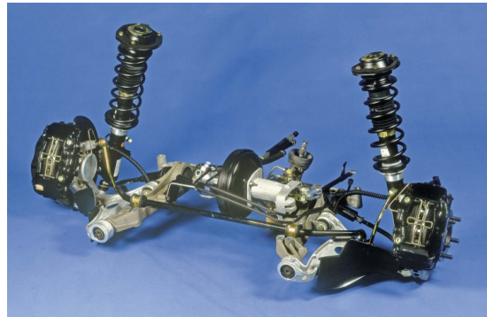
Front suspension, along with the brakes and steering set-up. The forthcoming Carrera 4 version would naturally include a differential and driveshafts.
