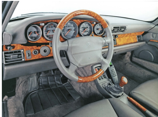
A 993 coupé with the wood and leather options from the Exclusive catalogue. Note the red-line on the tachometer, marked at 6800rpm, just before the cut-out was set to activate.
