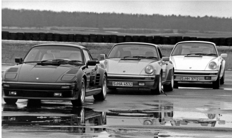
The mighty Turbo, seen here in slant-nose guise (left) and regular coupé form (centre). A standard 3.2 litre Carrera is bringing up the rear, providing an ideal view of the different wing profiles used on the turbocharged and NA cars, and the unique panels employed on the flat-nose conversions.
