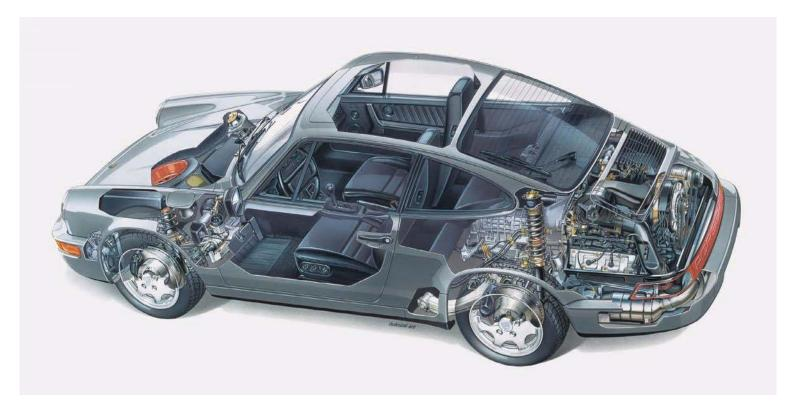
to be split between front and rear wheels, increasing the stability under all conditions. The downside was increased weight and greater complexity.
