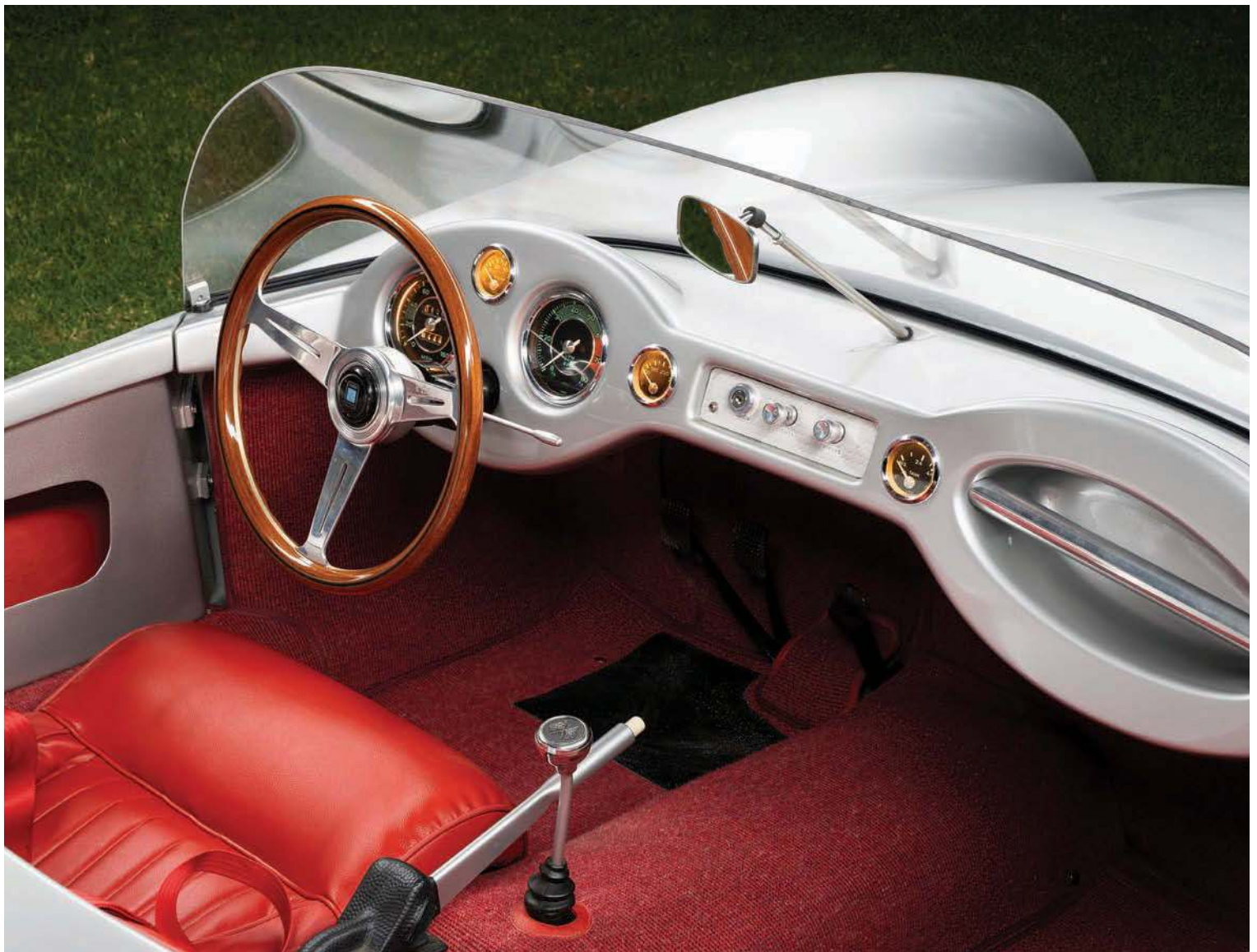
Above: Dashboard carries auxiliary gauges from North Hollywood Speedometer, alongside a very rare 356B Carrera speedo. Steering wheel is a Nardi Volante
