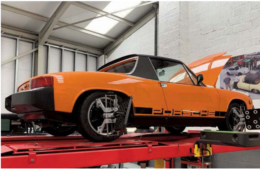
Above left: Suspension geometry was wildly out when the car arrived in the UK, so we had the car properly aligned using a four-wheel laser system at Williams-Crawford
