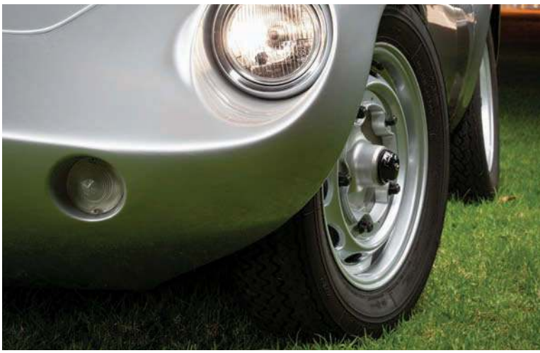
Above left: Wheels currently fitted are TechnoMagnesio, ultra-light rims in the style of the original Porsche wheels
