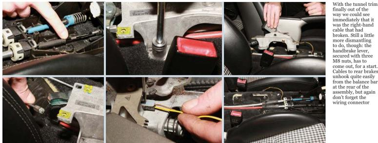
finally out of the way we could see immediately that it was the right-hand cable that had broken. Still a little more dismantling to do, though: the handbrake lever, secured with three M8 nuts, has to come out, for a start. Cables to rear brakes unhook quite easily from the balance bar at the rear of the assembly, but again don't forget the
