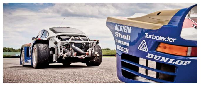
The 961 might have looked like a 959, but it was a far simpler device. The four wheel drive system remained, but the engine reverted to a basic, twin-turbo spec, swapping the road car's driveability for sheer 680bhp power
