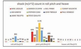
Industry engineers conclude the driver is more sensitive to roll and pitch shocks. The driver is further sensitive to pitch (fore-aft of nod) or, if you like, the fore-aft swing of the fluffy dice hanging from the rear view mirror.
