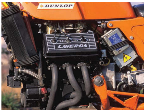
ABOVE: The V6 was a scaled down 4-valve development of the Maserati Merak engine
