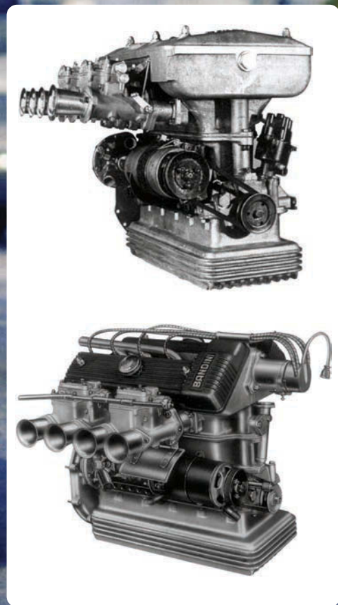
TOP: Twin-cam 750 engine based on a Crosley block ABOVE: Second version with developed head
