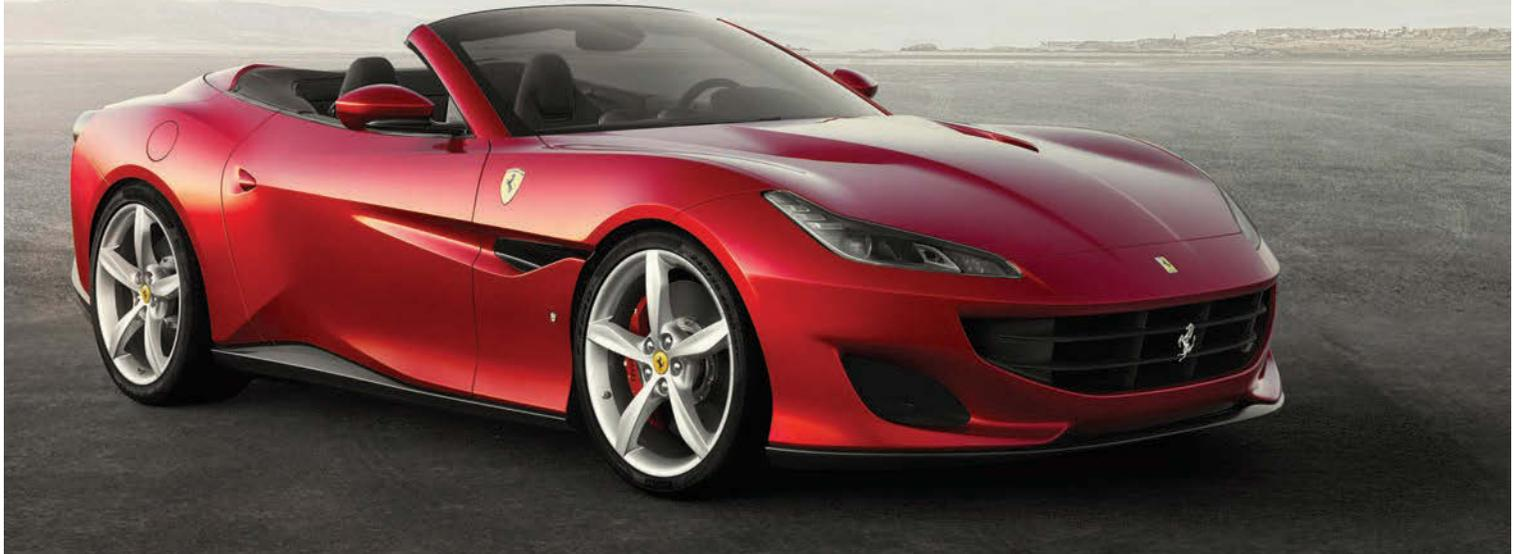
The chassis is all-new, featuring lower weight than the California T and increased torsional rigidity. Ferrari's third-generation electronic rear differential (E-Diff3) is adopted, while the Portofino also becomes Ferrari's first GT to be fitted with electric power steering, enabling a faster steering ratio. The damping system has been updated, too, reducing roll and improving bump absorption.
