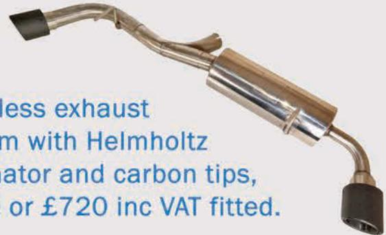
Stainless exhaust system with Helmholtz resonator and carbon tips,
