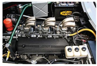
The spec of the V12 echoed that of the 250 LM but in the larger 275 size, delivering over 300hp
