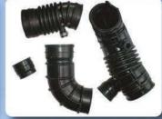
TS and V6 intake rubber pipes are a specialty. It is a part that often needs to be replaced on cars getting on for 20 years old and as we have had them made in large quantities, should have them available for the next 20 years! 3.0 and 3.2 intake runner pipes also made exclusively for us.
