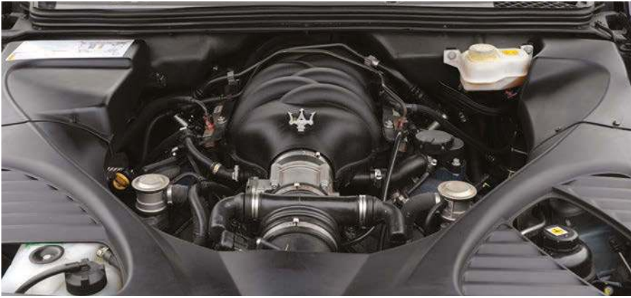
Bellagio uses superb 4.2 V8 engine (above). Model chosen for the QP6 estate was a 275hp diesel (below)
