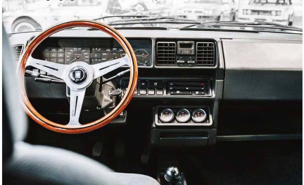
BELOW: Interior boasts a Nardi steering wheel with a wooden rim and three extra Veglia gauges housed in the radio compartment
