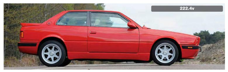
The standard Biturbo package was potent, but it's not the Italian way to settle for merely potent; faster is always better. The early go-faster Biturbo was the 'S', which first introduced intercooling to the model – and nifty NACA ducts to the bonnet. Designed for the Italian market, it packed 205hp compared to the standard car's 185hp, and featured stiffer suspension, two-tone bodywork and wider tyres.
