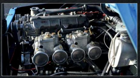
decided to build a 1300 unit based on the Fiat/Lancia 1300, as used in home-market Fiats and Lancia Deltas. This is a super engine with the same crank journal sizes as a 2.0-litre unit and produces around 80hp on a single carburettor. It's a really robust power unit whose bore and stroke of 86.4mmx55.5mm are extraordinarily close to Abarth's 86mmx55mm.
