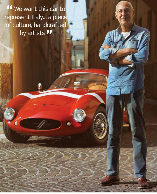
sketched out in advance. Leonardo explains: "There is no design. We used craftsmen with the ability to weld and shape a framework of tubes and then cover it in aluminium, all done by eye. We created the body in the metal first and only then scanned it. You could say we started at the end first!"
