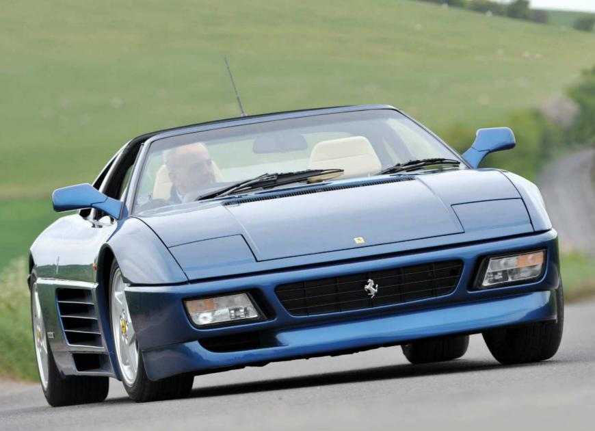
The 348 marked a new direction for Ferrari in that it abandoned spaceframe construction for a body formed of box sections, giving it 50 per cent greater torsional rigidity. The 348 tb was heavier than the old 328, tipping the scales at 1393kg (versus 1263kg). Yet its V8 engine had only 30hp more power and 15lb ft extra torque: the 348 had 300hp on launch (later upped to 320hp).
