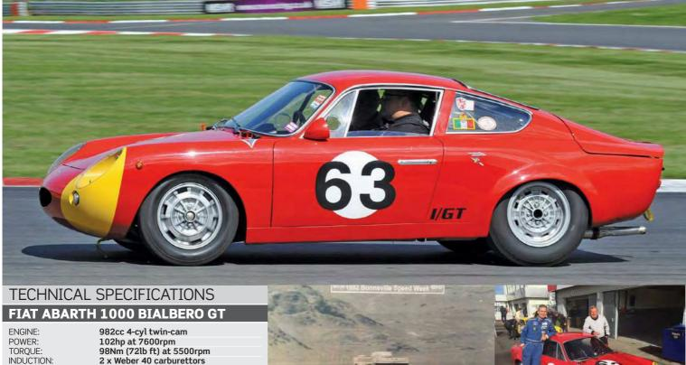
ENGINE: POWER: TORQUE: INDUCTION: TRANSMISSION: BRAKES: DIMENSIONS: WEIGHT: MAX SPEED: 982cc 4-cyl twin-cam 102hp at 7600rpm 98Nm (72lb ft) at 5500rpm 2 x Weber 40 carburettors 5-speed manual Discs front & rear 3470mm (L), 1350mm (W), 1110mm (H) 560kg 121.779mph
