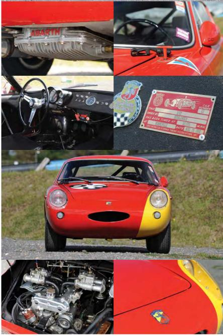
dampers, Girling disc brakes and Campagnolo wheels were the major additions to the Fiat chassis. The gearbox was an Abarth five-speed unit based on the Fiat 600D transaxle, which offered a wide variety of gear ratios and final drives.
