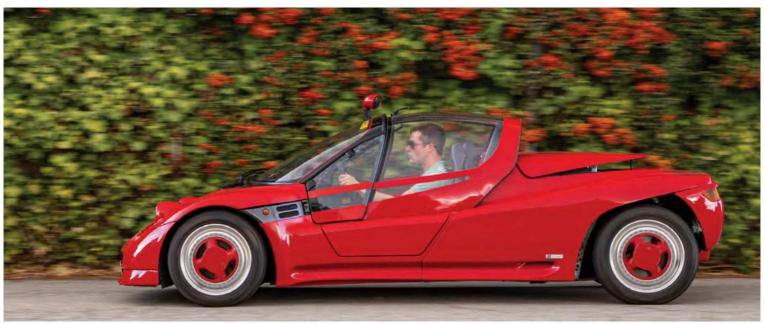
Radical design underpinned by pioneering carbonfibre honeycomb chassis, pushrod suspension, transaxle
