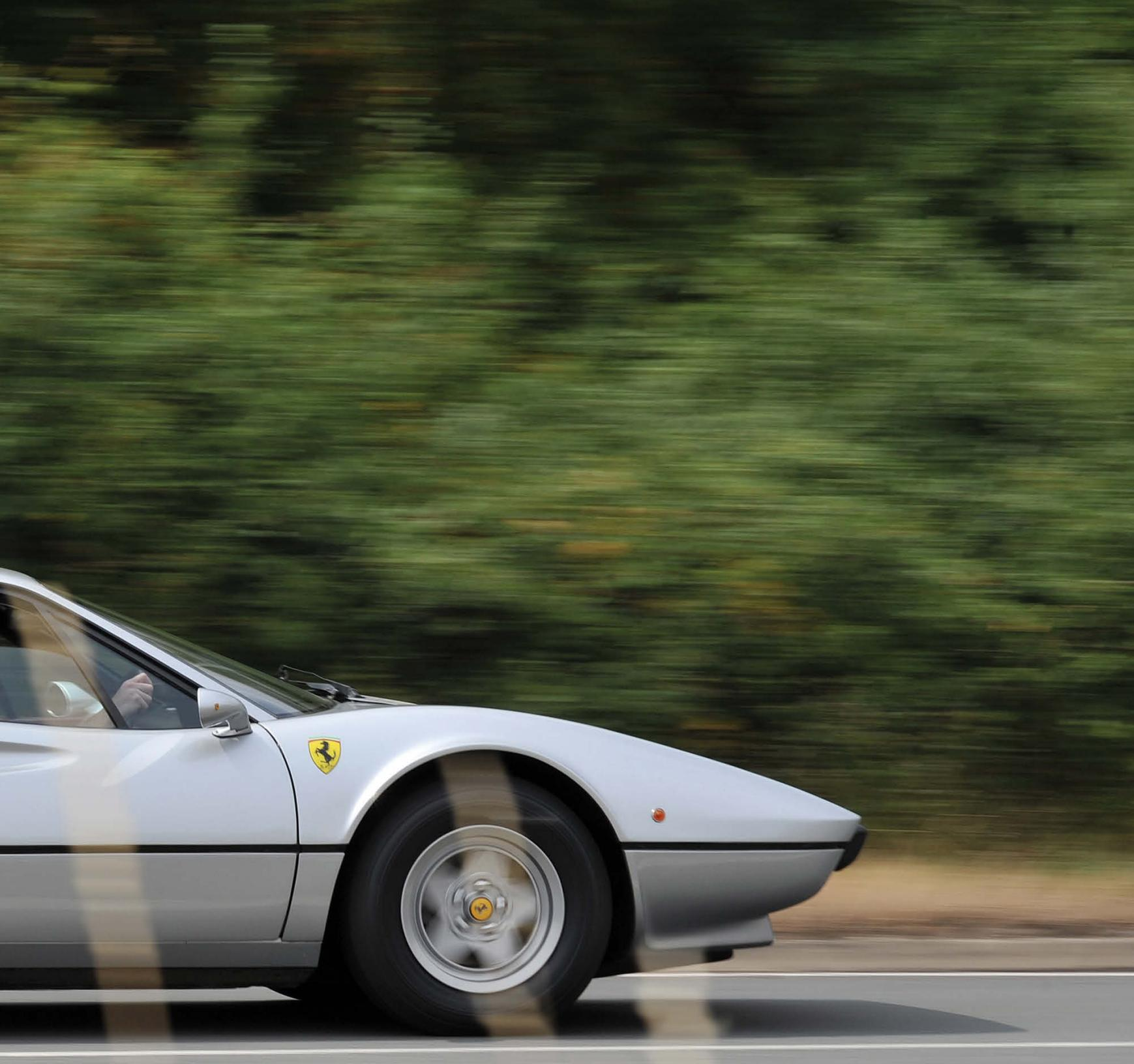
documented – perhaps it caught wind of the rival Lotus Esprit, also revealed at the Paris Motor Show in 1975 – but ‘adding lightness’ was certainly a consideration. Hung on a tubular steel chassis, the plastic body and panels – excepting the aluminium front lid – resulted in a dry weight of just 1090kg. Add around 100kg for the ‘DIN’ kerb weight figure, including fluids and a 90 percent tank of fuel, and this V8-engined Ferrari is still lighter than many of today’s three-cylinder superminis.
