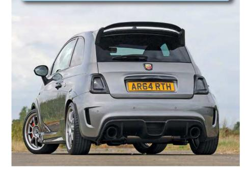
passengers in the rear. Its MTA automated manual gearbox has a TCU map as well as an ECU remap that give a much snappier response in both paddleshift and automatic modes. Personalisation options include OZ alloy wheels finished in shadow chrome wrapped in Michelin Pilot Sport 4 tyres.
