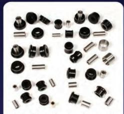
It came to light that there are two size options on the rear spring pan arm outer bush, so we offer both shell size options 39.9 & 42.2 mm OD, so please be aware of this option when ordering. The spring pan arm outer bushes are designed to rock as the original greased steel ball, whilst minimising radial movement – hence the hour glass profile & suitable stainless shell. The sharp edges of the arm housing would be detrimental to a conventional flanged bush.
