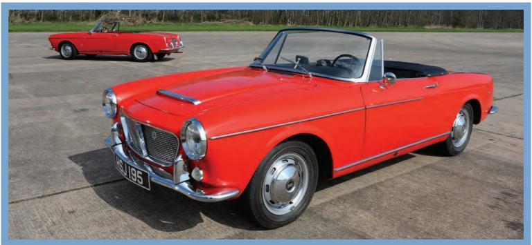
despite having a mere 83bhp at the crank, it feels a lively, tough and torquey engine. No, it's hardly the last word in sportscar performance off the line, but it'll happily pull along at motorway speeds. It shares its five-speed gearbox with the Fiat 124, but does suffer from a 'whippy' canted gear lever that can be a little awkward to engage.
