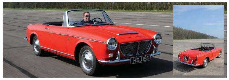
ABOVE: This 1200 Cabriolet has the most original specification of the group having a 'relaxed' 55bhp And it sounds great, too, helped by a stainless steel replica of the original OSCA exhaust system. The fivespeed gearbox (five ratios – very fancy for the time) works well, too, the lever slotting positively into each position in its gate.
